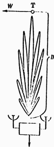
Figure 37. Principle involved in the use of a radio interferometer to measure speed and distance.
