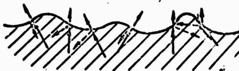
Figure 4. Reflection from the inner surface of a non-flat radiator.
