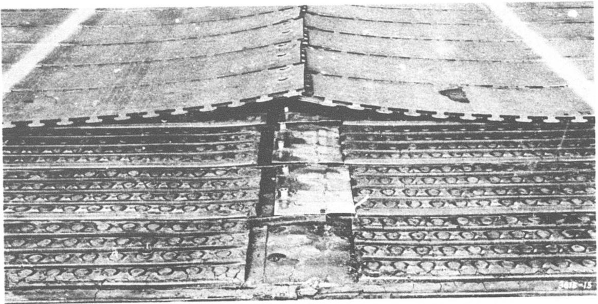
Fig. 8. Sheared end plates after six coverages
