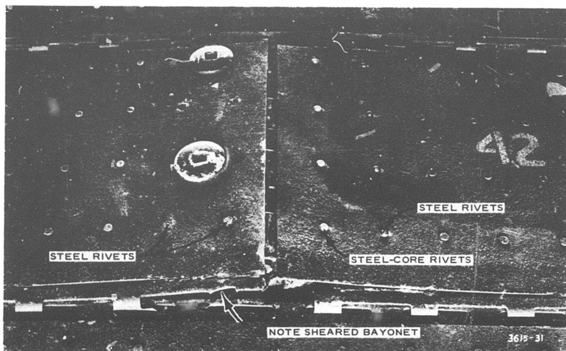
Fig. 9. Condition of steel rivets in plank after 78 coverages.
