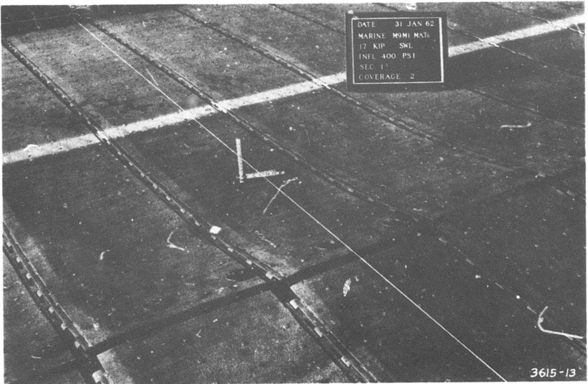
Photograph 1. Item 1 after 2 coverages had caused end joints to arch up
