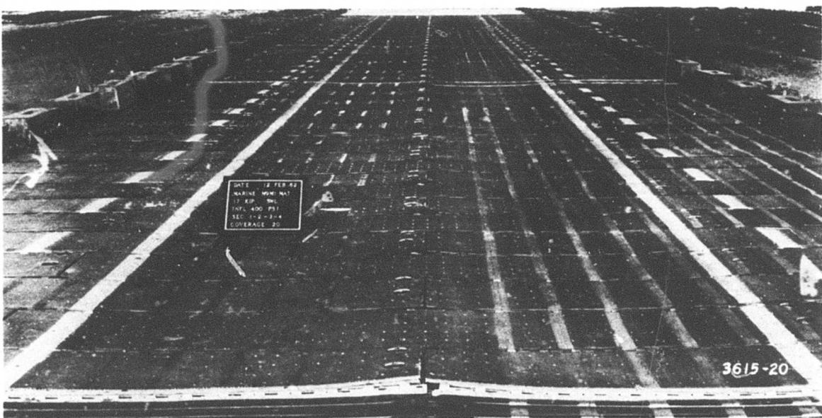
Photograph 4. Test section with staggered end joints after 20 coverages
