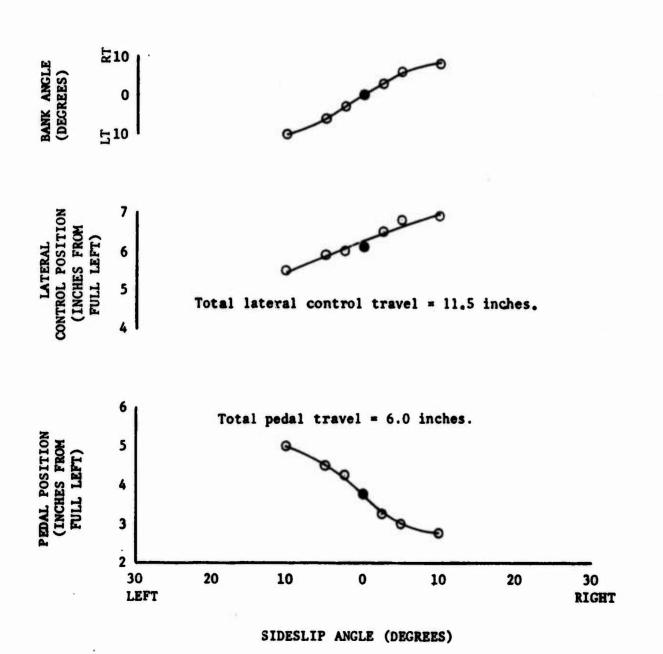
FIGURE 5 MANEUVERING STABILITY RV-1D/QUICK LCOK II USA S/N 67-18905
