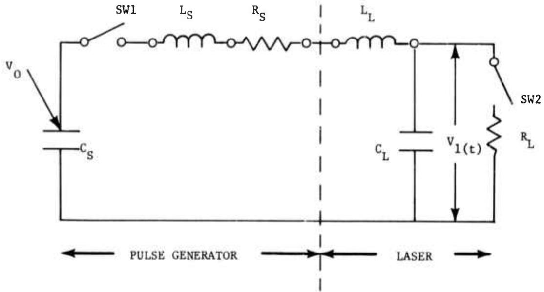
Figure 10. Equivalent Circuit of the Pulse Generator and Laser Discharge. The storage capacitance is  $C_S$ . The thyatron,  $SW1$ , is characterized, when conducting, by inductance,  $L_S$ , and resistance,  $R_S$ . The inductance and capacitance of the laser structure and the connection to the generator is denoted by  $L_L$ , and  $C_L$ , respectively. When breakdown occurs ( $SW2$  closed), the active medium is characterized by resistance  $R_L$ .
