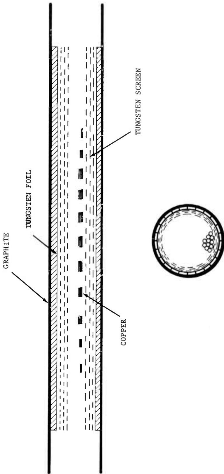
Figure 2. The Heat Pipe Cell
