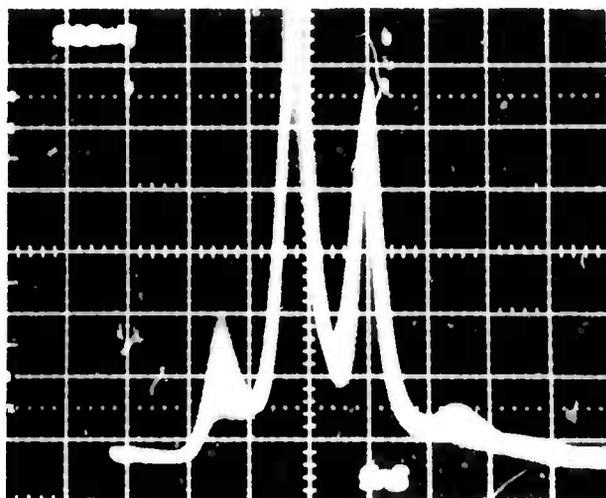
Figure 14. Oscilloscope Photograph Showing Multiple Laser Pulses. Vertical deflection:  $1.5 \text{ kW-div}^{-1}$ ; horizontal deflection:  $5 \times 10^{-9} \text{ sec-div}^{-1}$ . Wavelength is  $0.5106\mu$ .
