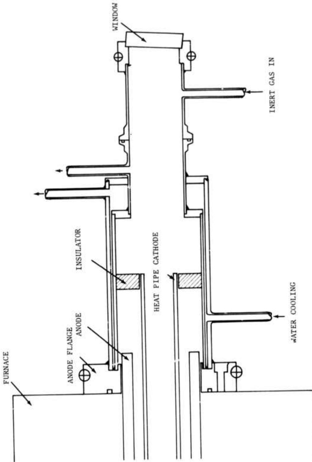
Figure 11. Output Window Flange Assembly
