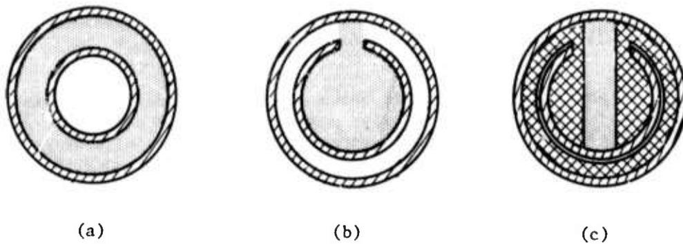
Figure 4. Cross Sectional Views of Transverse Discharge Electrode Configurations. The electrodes are the concentric cylinders indicated by the diagonal lines. The inner cylinder in each figure is the cathode. The regions in which the discharge occurs are shown as dotted in the figures. The cross-hatched region shown in (c) represents dielectric material.
