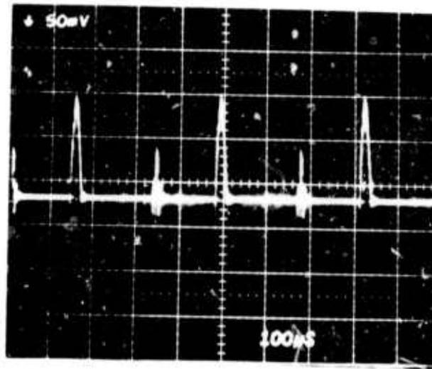
Figure 7. Operation of the Pulse Generator at  $3 \times 10^3$  pps. The large pulses (at 100 mv level) are three consecutive charging current pulses. The peak charging current is 1 A. The four smaller noise bursts, delayed from the charging pulses by 180  $\mu$ sec, are generated during the discharge of the storage capacitors into the laser electrode structure.
