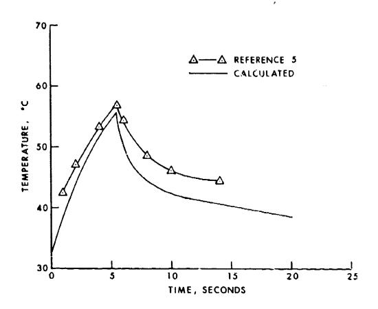
Figure 5. Calculated and Experimental Temperature Histories.
