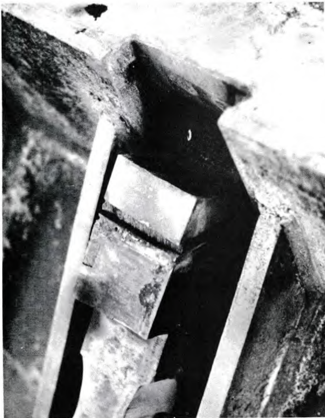
Figure 35. STATO anchor with plate addition between shank and wedge insert to reduce fluke angle to about 32 degrees.
