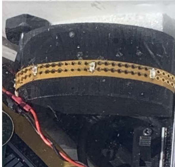
Figure 31. Array of Three Flat Phototransistors Attached to Arced Platform
