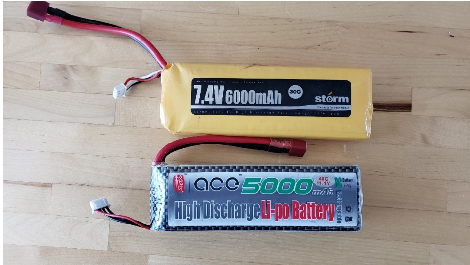
Figure 18. Transmitter and Receiver Batteries
