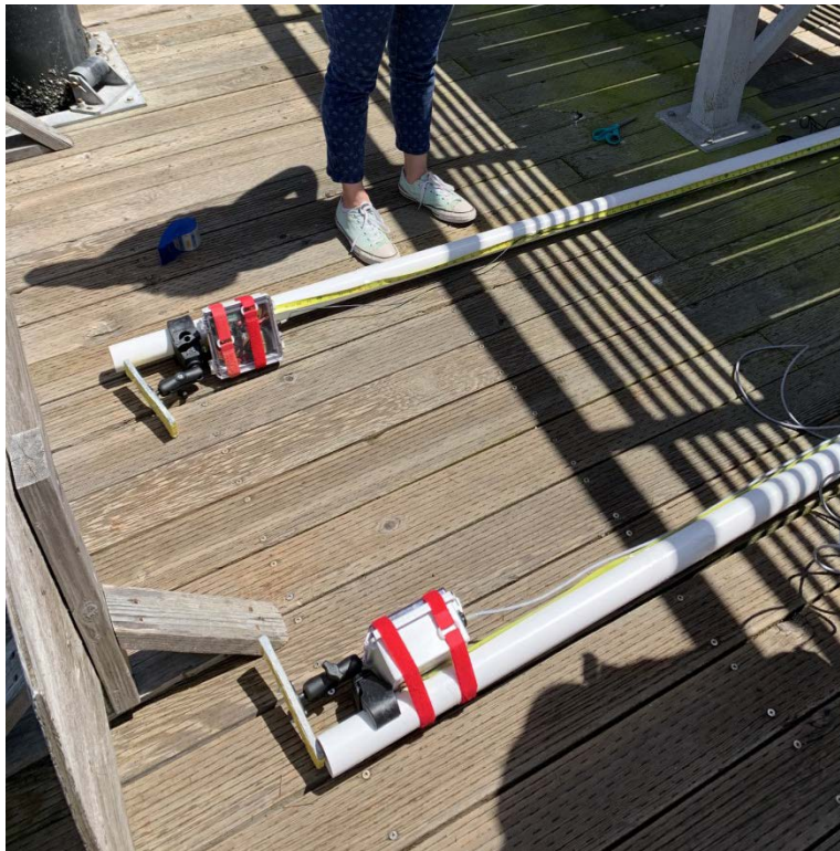
Figure 33. VLC Transmitter and Receiver Attached to PVC Pipes
