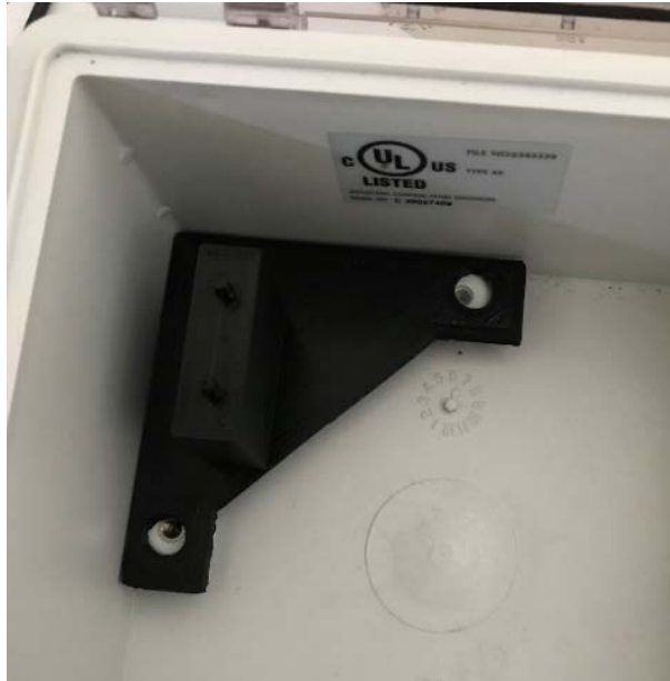
Figure 26. 3D Printed Platform for Arced Phototransistor Array
