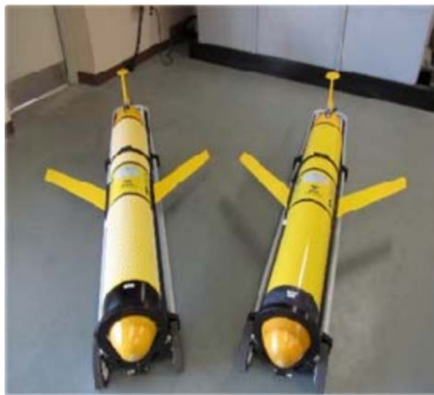
Figure 4. Littoral Battlespace Sensing—Unmanned Underwater Vehicles (LBS UUV). Source: Mensi et al. (2014).
