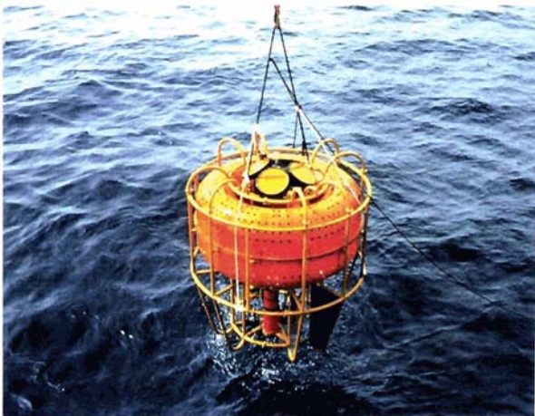
Acoustic doppler current profiler under launch.
