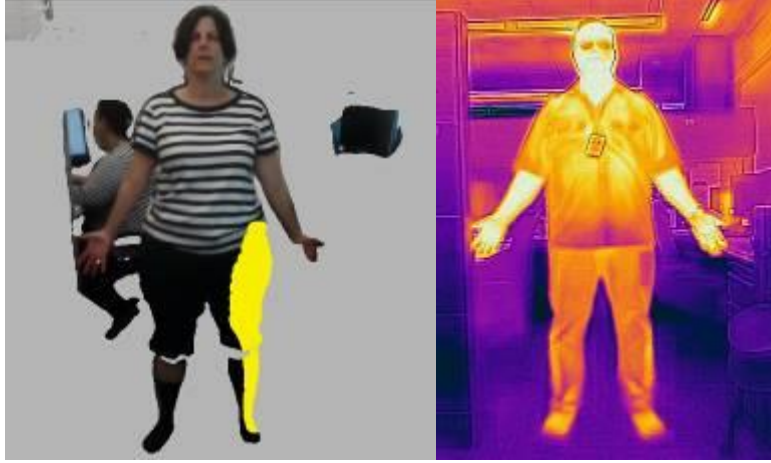
Figure 6. FLIR One Composite of thermal image mask and RGB image (left) and FLIR One Thermal Image (right).
