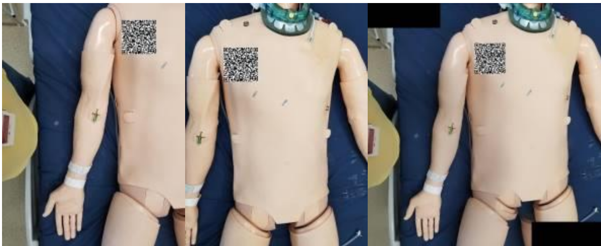
Figure 26. (LEFT) Mannequin arm with QRF marker, (CENTER) Mannequin trunk with marker, (RIGHT) images stitched together using OpenCV.
