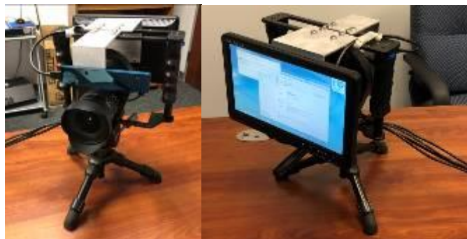
Figure 4. Our MSI platform combines a COTS MSI imager (large lens), Intel RealSense Depth camera (blue bar on front), and a touchscreen (left picture) into a portable device. This platform is tethered to a laptop that is required during data collection, but imaging is controlled via the integrated touchscreen and a custom Windows-based application.
