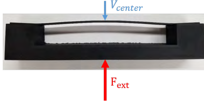
Fig. 2: 3D-printed curved beam with base excitation shown and response .
