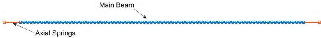
Fig. 63: Finite element model representing the nominally flat beam as flat with axial springs representing the boundary stiffness.
