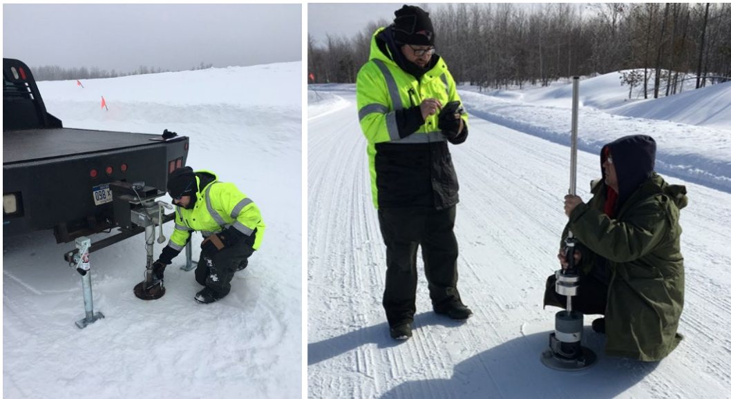
Figure 2. Field CBR (left) and LWD (right) tests Michigan.
