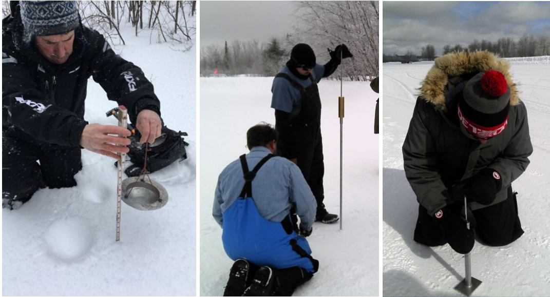
Figure 1. Yamaha drop cone (left), Rammsonde (middle), and CTI (right) tests in Michigan.
