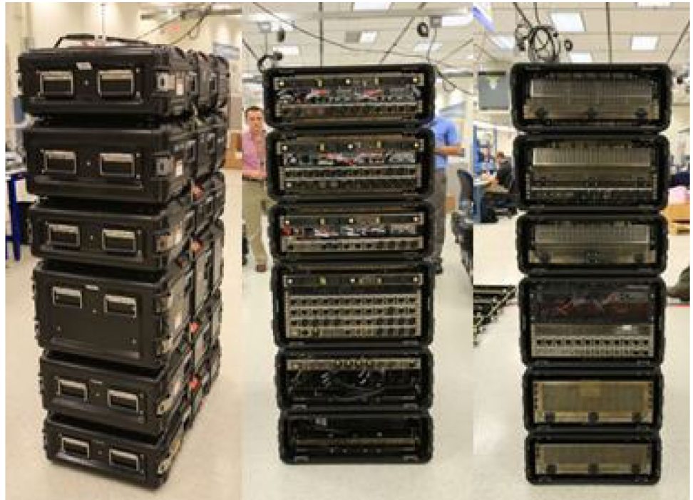
Figure 7: A Standard Operating Unit in Its Transportable Casings (left), the Back (Center) and the Front (Right) of An Uncased Unit
