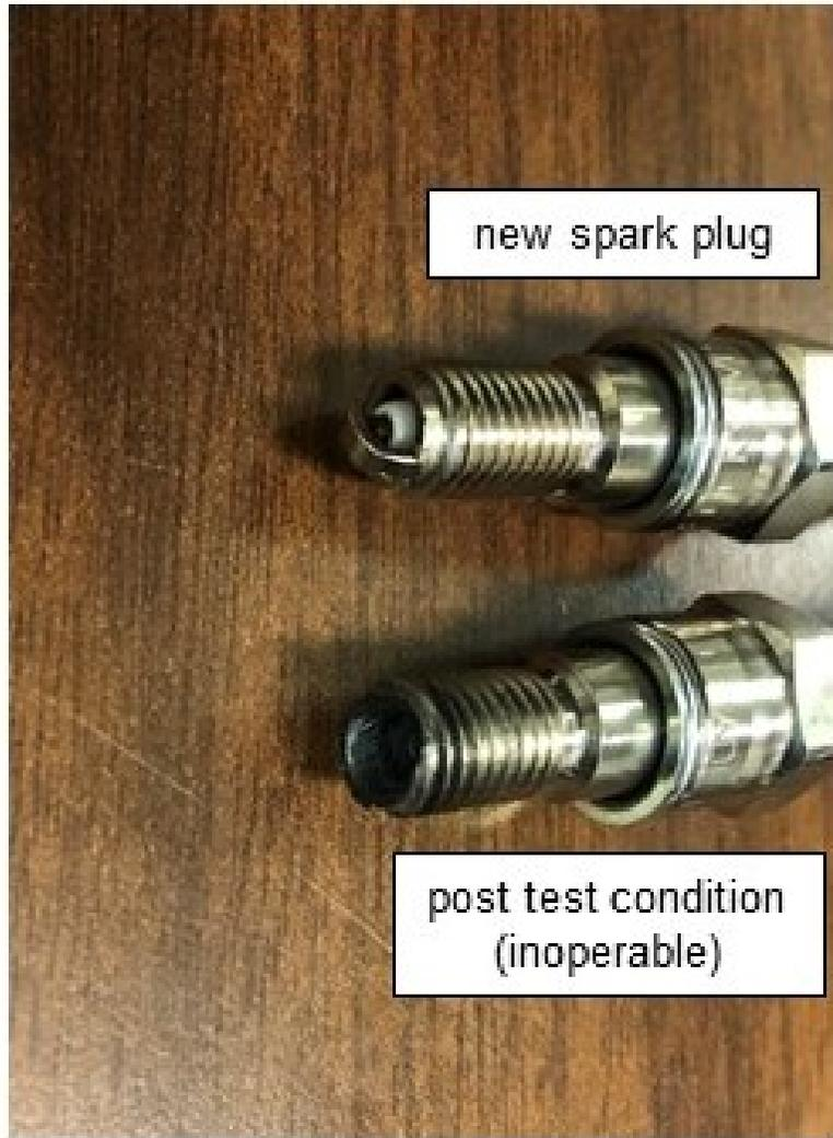
**Figure 73. Spark plug condition pre and post testing**
