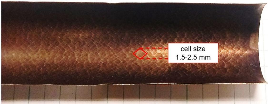
**Figure 26.** Soot foil used to determine cell size of  $C_2H_6$  and  $N_2O$  at  $\phi = 1.0$  courtesy of Sell et al.
