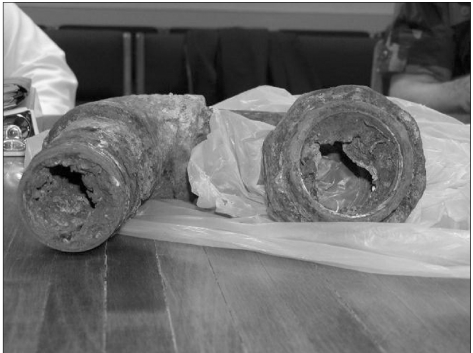
Figure 6: Choked and Clogged Water Pipes at Pope Air Force Base, North Carolina
