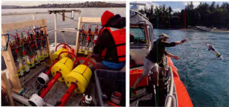
Figure 2. Left: uFloats and DAISys on deck for deployment. Right: uFloat during deployment in Sequim Bay, WA.
