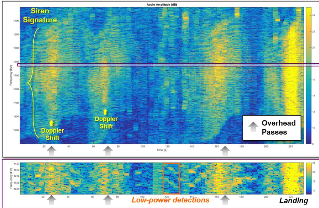
Figure 18. Siren audio signature during flight testing.
