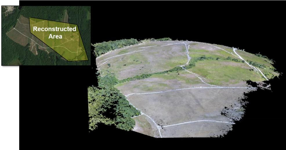
*Figure 14. Structure-from-motion 3D reconstruction of Turner Drop Zone at Fort Devens.*
