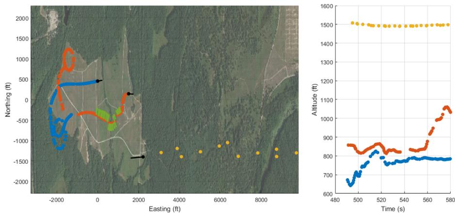
Figure 29. First encounter with the manned aircraft. Blue and red dots denote position of sUAS from telemetry. Yellow dots denote the manned aircraft track from the radar feed.
