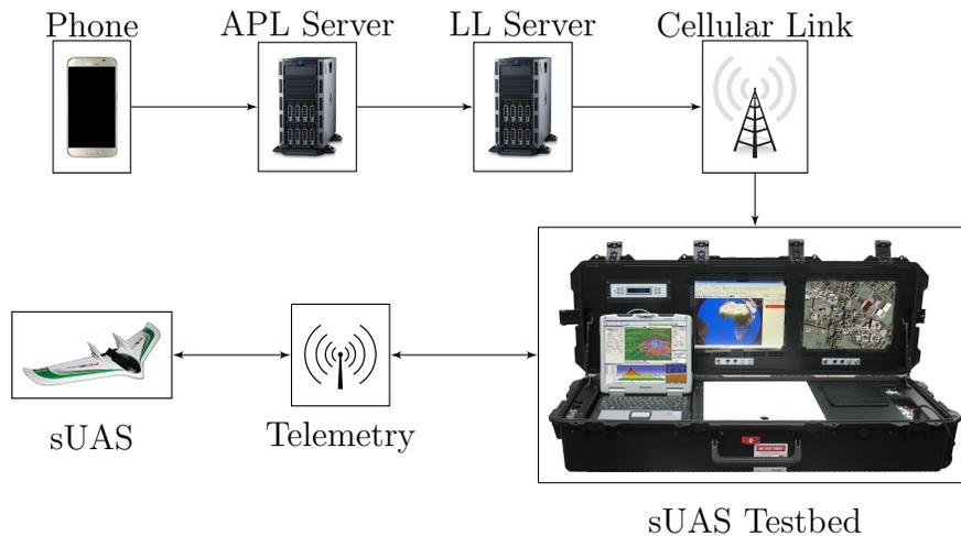
Figure 26. Phone with Cloud-based surveillance.
