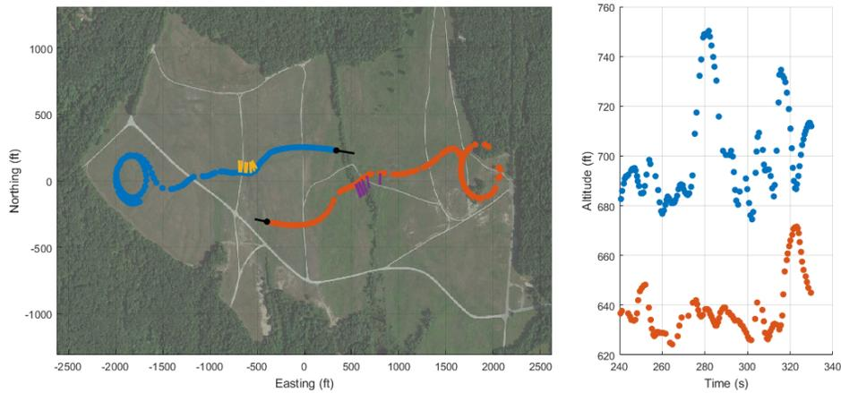
Figure 32. Encounter between two unmanned aircraft both equipped with collision avoidance logic. Collision avoidance advisories are displayed as yellow and purple arrows on the tracks.
