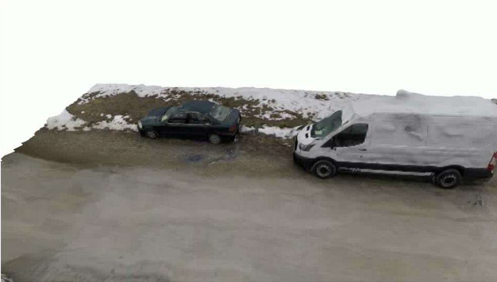
*Figure 15. Structure-from-motion 3D reconstruction of Vehicles.*
