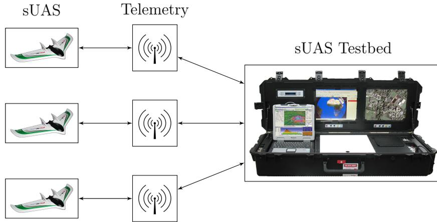
Figure 25. Shared telemetry surveillance.
