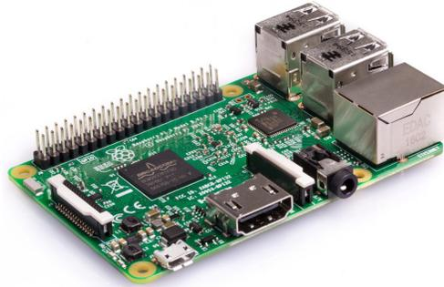
*Figure 10. Raspberry Pi 3 Model B.*
