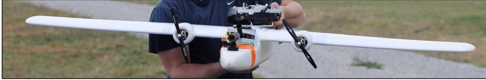
Figure 17. Siren as mounted on MTD test platform.
