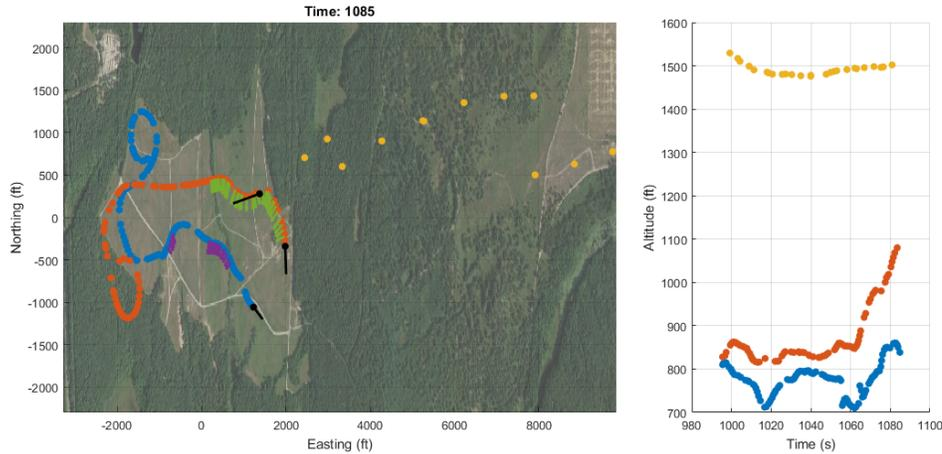
Figure 30. Second encounter with the manned aircraft. Blue and red dots denote position of sUAS from telemetry. Yellow dots denote the manned aircraft track from the radar feed.
