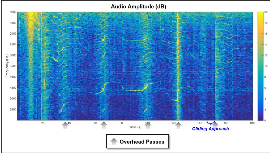
Figure 20. Acoustic signature of FX-61 motor.
