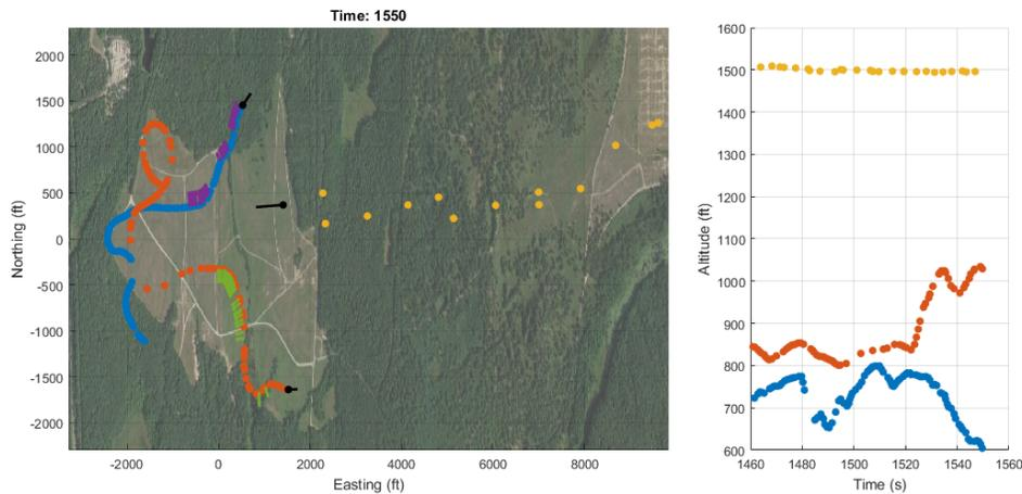
Figure 31. Third encounter with manned aircraft. Blue and red dots denote position of sUAS from telemetry. Yellow dots denote the manned aircraft track from the radar feed.
