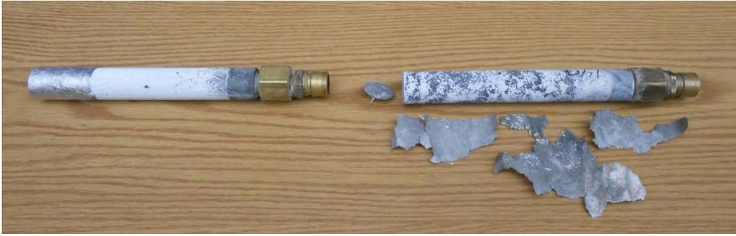
**Figure 4.2.2: Post Dunker Aluminum Coating Adhesion test**
