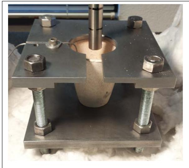
**Figure 3.2.2:** Experimental set-up for pull-out test
