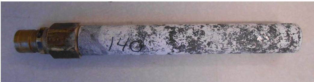
**Figure 4.2.1(a): One Coat 140 Cycles**
