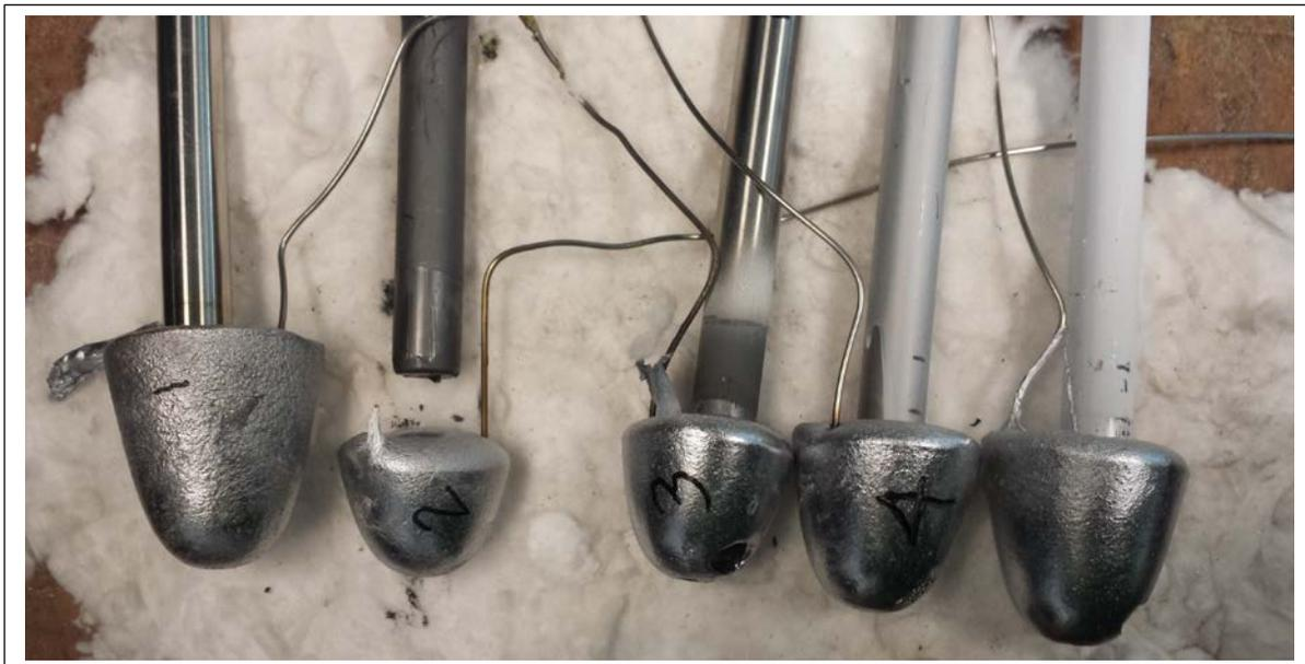
**Figure 4.1.1:** Tested specimens showing the coated rods and aluminum slugs
