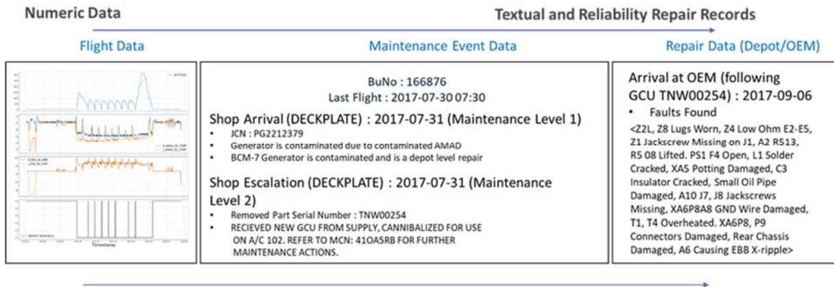
Figure 3-3. Correlation of Data Across Sustainment Process for Specific GCU Serial Number
