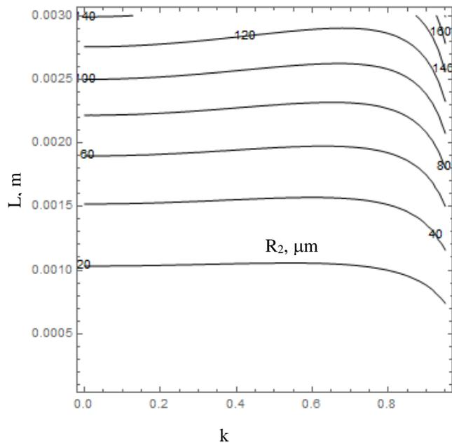
**Fig.9:** External radius  $R_2$  as a function of  $k=R_2/R_1$  and the length of the cantilever
