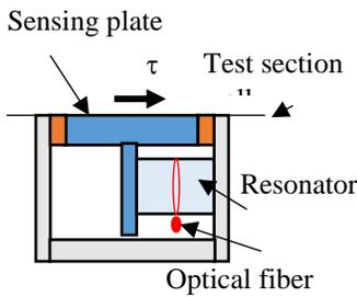
**Fig.3:** Schematic of the 1D skin friction sensor
