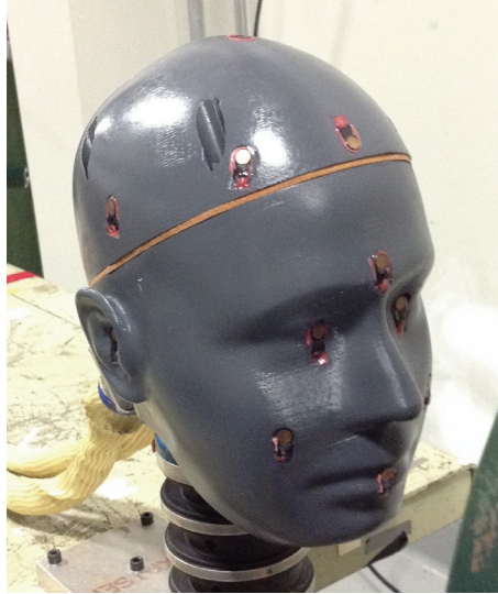
Figure 5.11. Basic Human Surrogate Head Model
