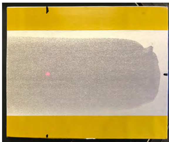
Figure 10. 75 \mu\text{m} layer of plain Al-Si-10Mg powder manually spread on Al-12Si substrate with a beveled steel blade.
