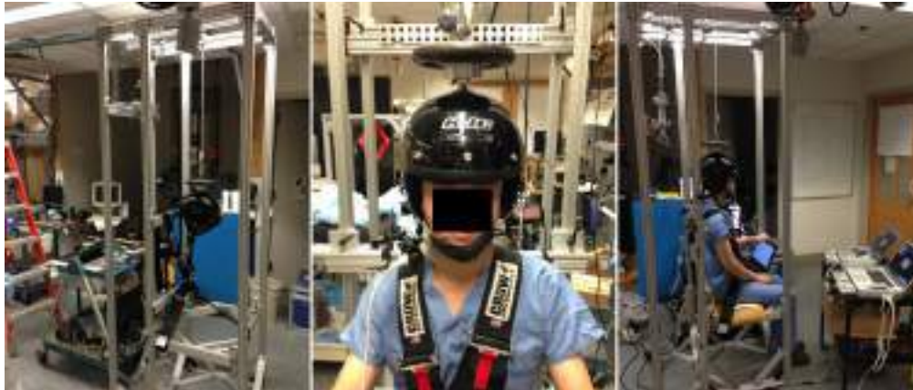
Figure 1-23: (left) Solenoid powered traction system for applying cyclic loads in-vivo : a programmable DC power supply is used to power a solenoid that applies a variable traction force via two fixed pulleys to a fixed weight attached to the top of the helmet; (middle) front view; (right) a side view demonstrating restraints and dual ultrasound probes positioned on the subjects neck anteriorly and posteriorly in a fixed orientation.
