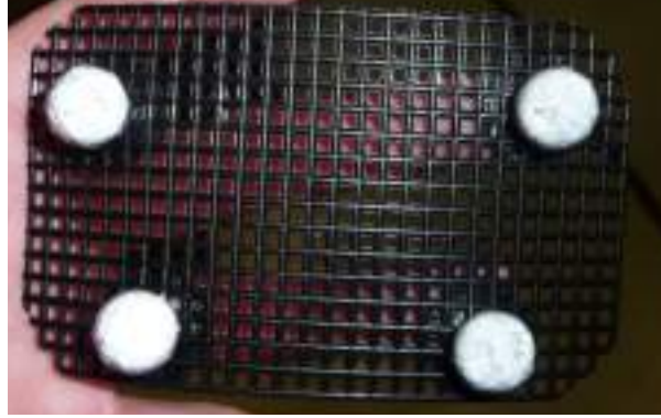
Figure 5-18: Example of a Vicon marker cluster.
