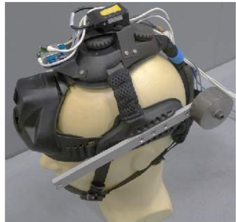
Figure 5-20: Skull Mounting System (left). HMSD configured with example rearward mass (right).
