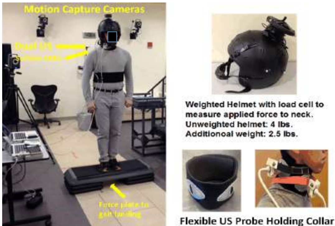
Figure 4-10: A volunteer performed a repetitive jumping test wearing a weighted helmet to simulate night vision/communication unit gear. Impact to the head and trunk during landing was measured by interposed helmet load cell and force plate. Resultant C4-C5 FSU deformation was measured by dual US system in real time. Para-cervical muscle (SCM, upper trapezius) activation was measured by surface EMG.
