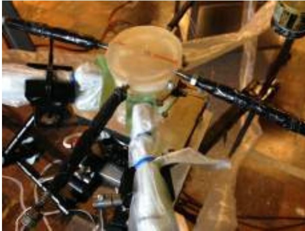
Figure 1-9: Lower vertebral body of the FSU mounted in PMMA and attached to a plate fixed on a tripod. Four hydraulic pistons rigidly attached to the PMMA allow the application of force couples that induced pure flexion-extension or lateral bending moments to the FSU. Dual US probes were oriented to image the facet joints and spinous processes of the C6-7 FSU.
