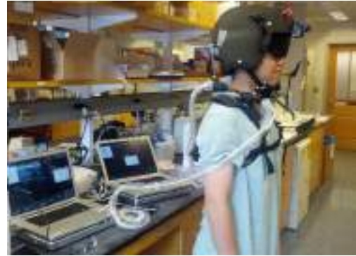
Figure 1-18: Dual US system on subject wearing army helmet.
