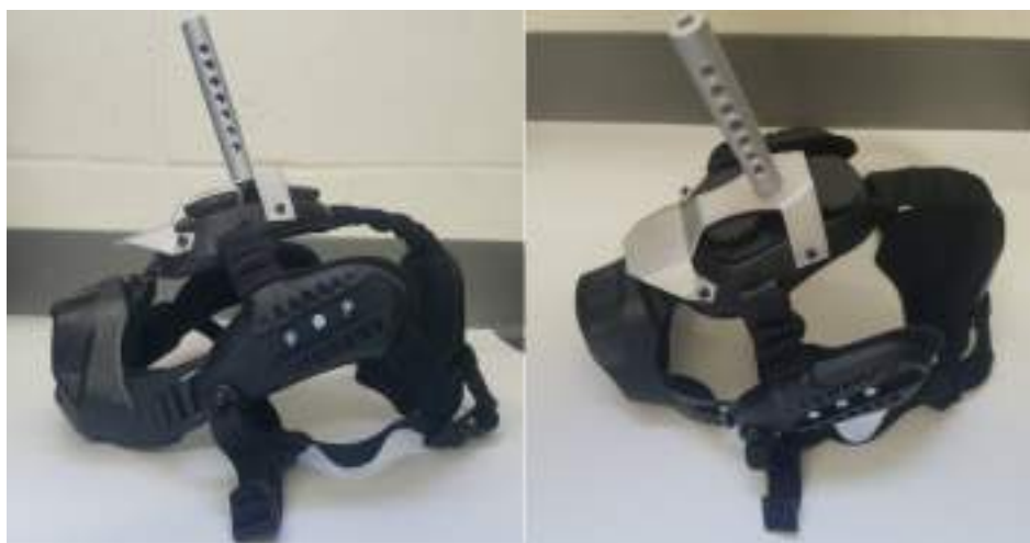
Figure 6-12: Helmet mass attachment device to recreate vertical (z-axis) offset helmet configurations.
