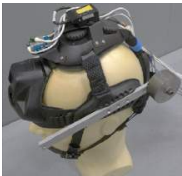
Figure 6-14: Helmet mass attachment device to recreate longitudinal (x-axis) offset helmet configurations.
