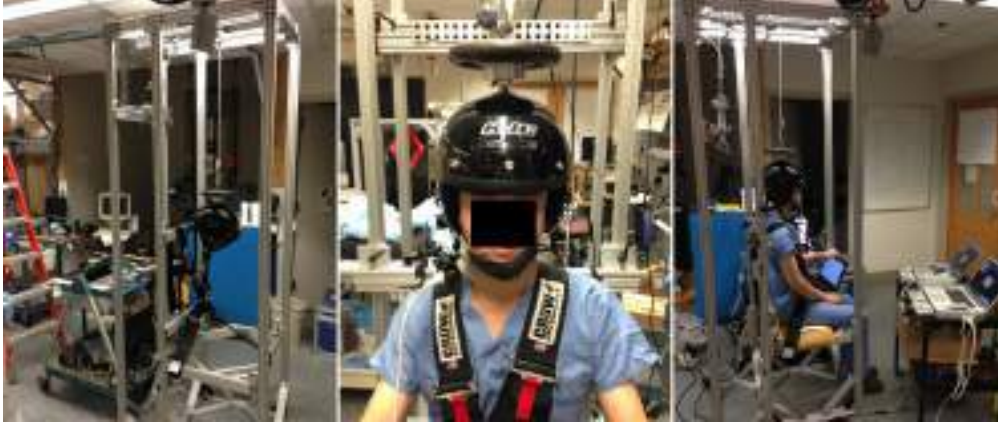
Figure 2-8: Solenoid powered traction system for applying cyclic loads in-vivo.
