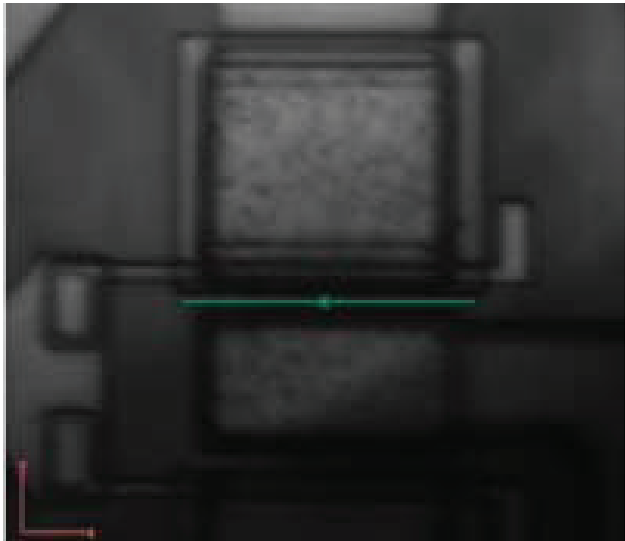
Figure 6. The target of the gate-drain gap irradiation.
