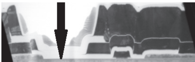
Figure 7. Transmission electron microscope cross section showing gate-drain gap target.
