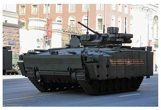
Figure E.3 **Epoch "Universal Combat Module" Remote Turret on Kurganetz-25**
