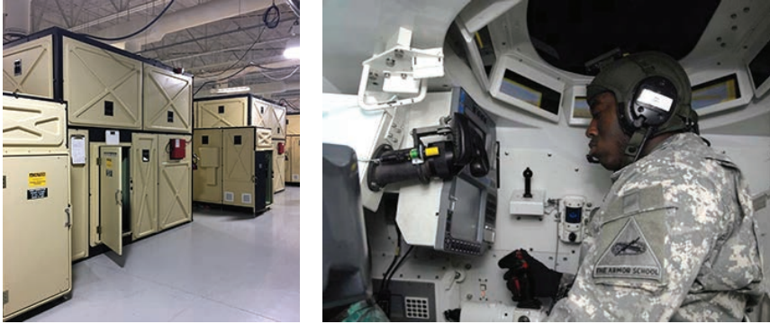
Figure 2.1 Exterior and Interior of Close Combat Tactical Trainer Manned Crew Modules
