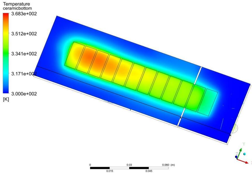
Figure 4. Temperature profile with two baffles. Baffles can be seen between the 2<sup>nd</sup> and 3<sup>rd</sup> diode from the right.
