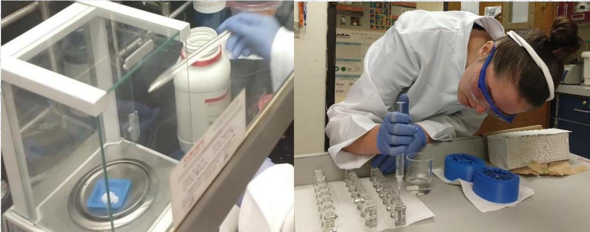
Figure 6. Student synthesizing PAA (left) and filling disk molds with PAA solution (right)
