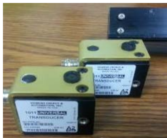
Figure 5.9. Temporary Installed Ultrasonic Meter and Its Accessories.
