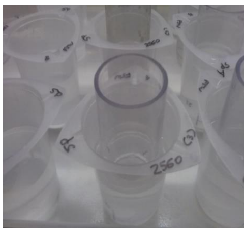
Figure 2-4. Test set up for sea urchin embryo exposures.
