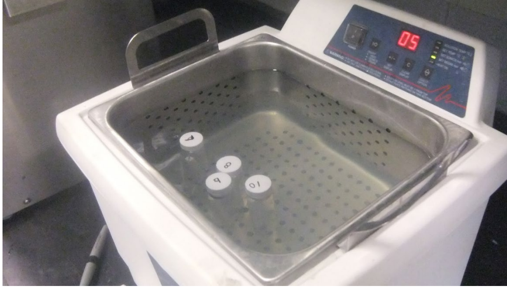
Fig. 6 Sonicator bath with glass vials containing each specimen
