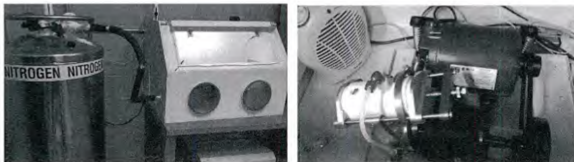
Figure 1 - Cryogenic milling apparatus with associated modifications to improve operational reliability and processing control.
