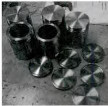
Figure 5 - Vials produced for low-contamination milling.
