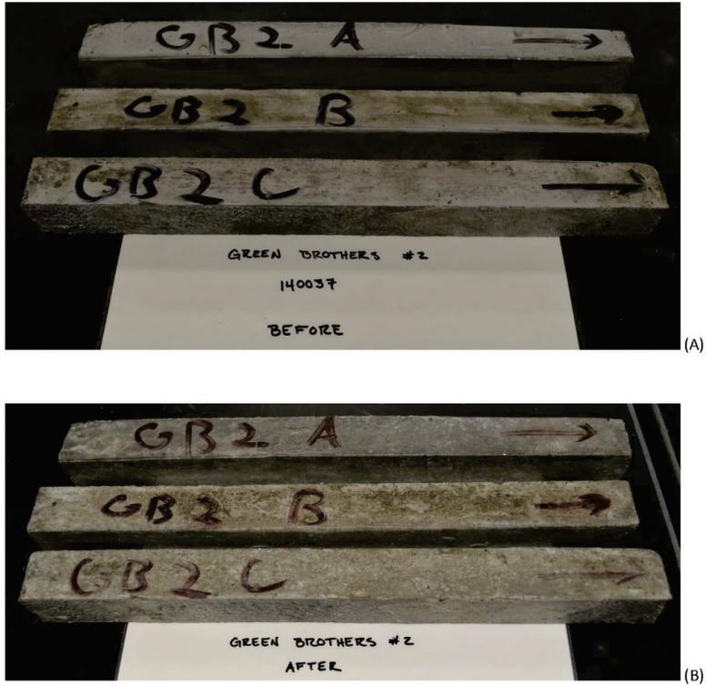
Figure A-9: Green Brothers #2 140037 (A) before autoclaving and (B) after autoclaving
