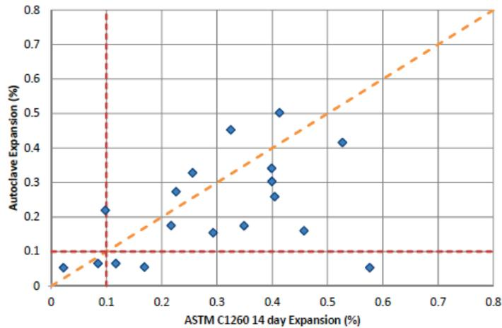
FIGURE 4: AUTOCLAVE EXPANSION RESULTS COMPARED TO ASTM C1260
