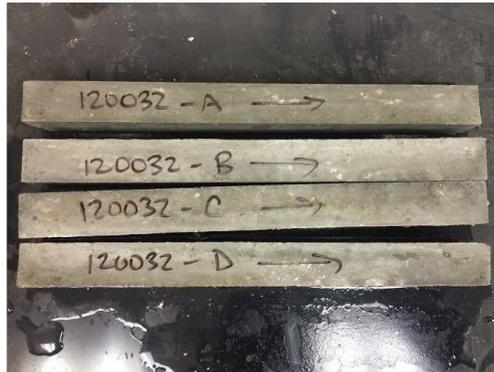
Aggregate 120032 Post Autoclave
