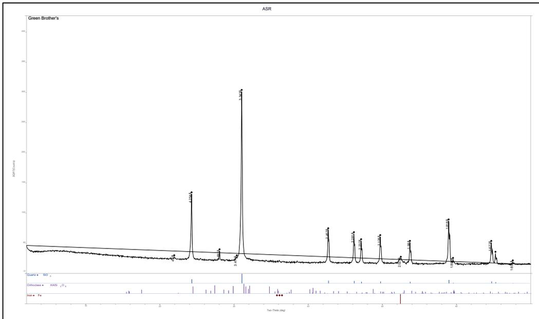
Figure B42. Whole pattern fit with mineral percentages Green Brothers Fine Aggregate Sample (CMB No. 130041).
