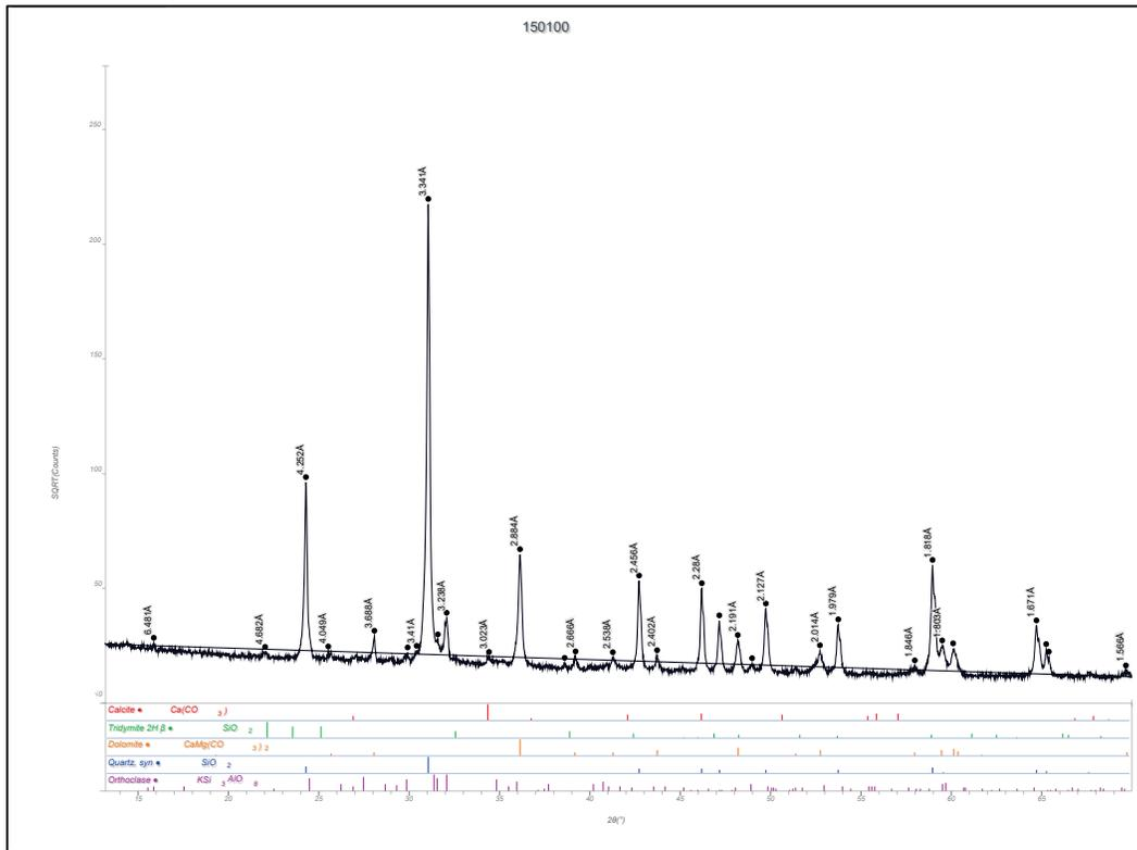
Figure B90. Whole pattern fit with mineral percentages Geneva, Utah, Coarse Aggregate Sample (CMB No. 150100).
