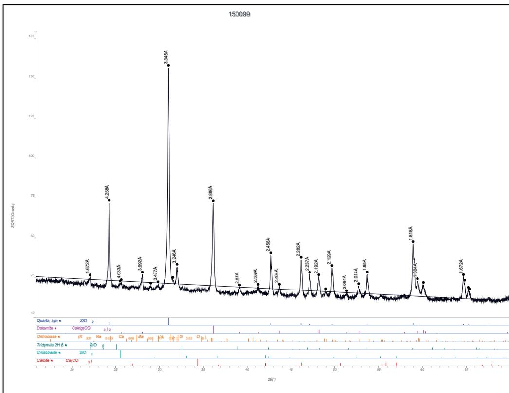
Figure B87. Whole pattern fit with mineral percentages Geneva, Utah, Fine Aggregate Sample (CMB No. 150099).
