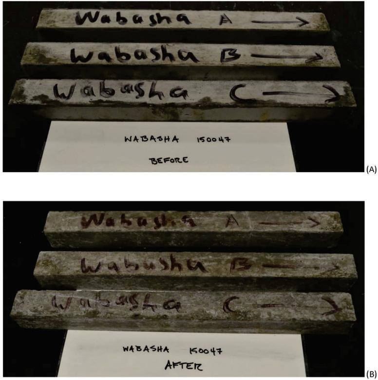
Figure A-10: Wabasha 150047 (A) before autoclaving and (B) after autoclaving
