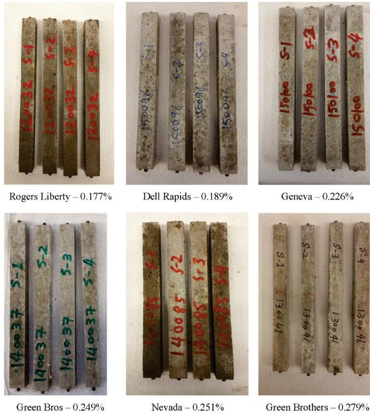
Figure 7 – Photographs of Mortar Bars Subjected to Autoclave Test (exp < 0.28%)
