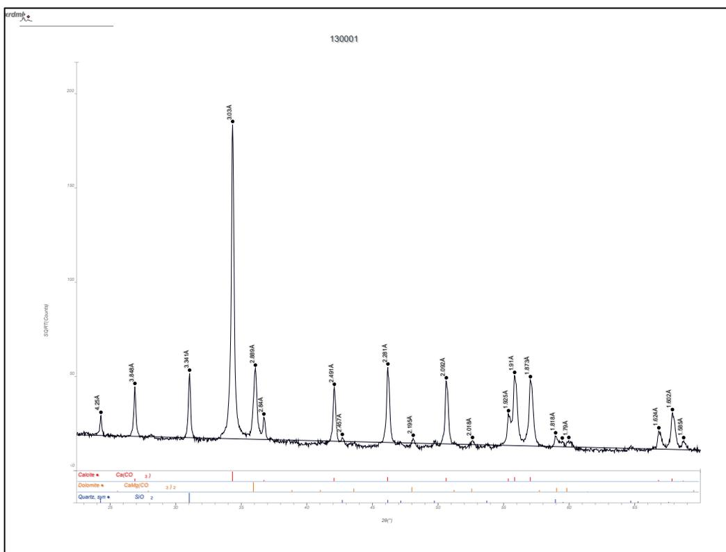
Figure B18. Whole pattern fit with mineral percentages Spratt Coarse Aggregate Sample (CMB No. 130001).
