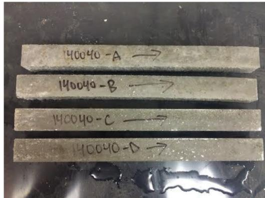
Aggregate 140040 Post Autoclave
