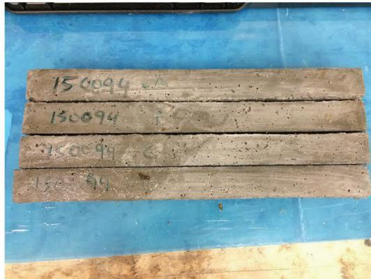
Aggregate 150094 Post Autoclave
