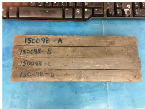
Aggregate 150098 Post Autoclave
