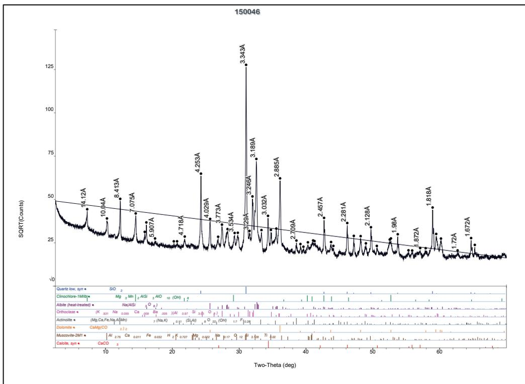
Figure B60. Whole pattern fit with mineral percentages Wabasha, MN, Coarse Aggregate Sample (CMB No. 150046).
