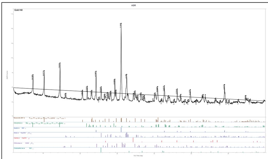
Figure B21. Whole pattern fit with mineral percentages NC Rhyolite Coarse Aggregate Sample (CMB No. 130002).
