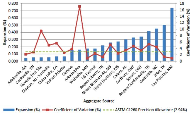
FIGURE 3: AVERAGE AUTOCLAVE EXPANSION OVERLAID WITH THE COEFFICIENT OF VARIATION BETWEEN EACH SAMPLE
