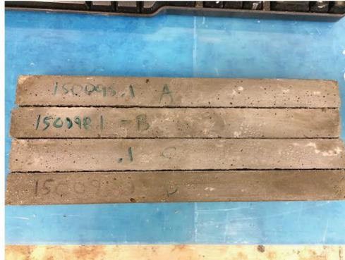
Aggregate 150098.1 Post Autoclave
