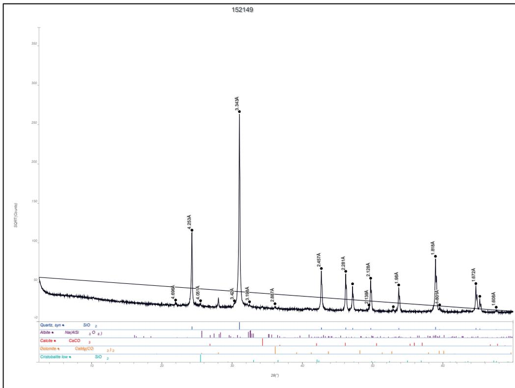
Figure B105. Whole pattern fit with mineral percentages Arkadelphia Fine Aggregate Sample (CMB No. 152149).
