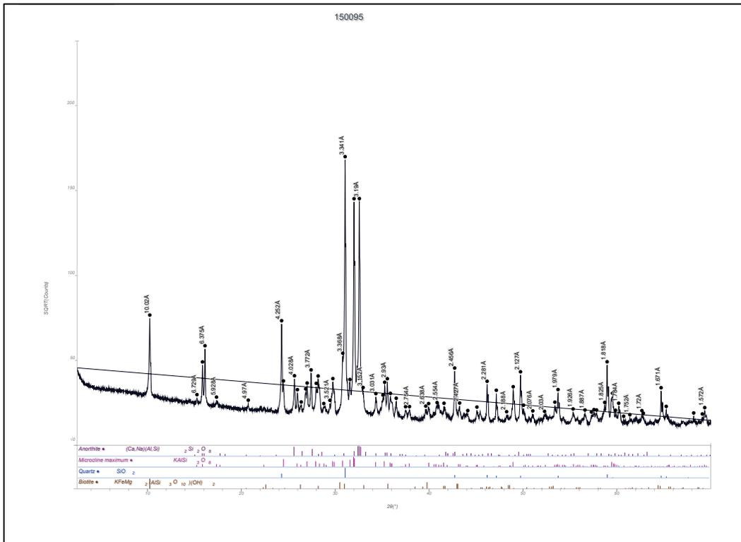
Figure B72. Whole pattern fit with mineral percentages Vulcan, Atlanta, GA, Coarse Aggregate Sample (CMB No. 150095).
