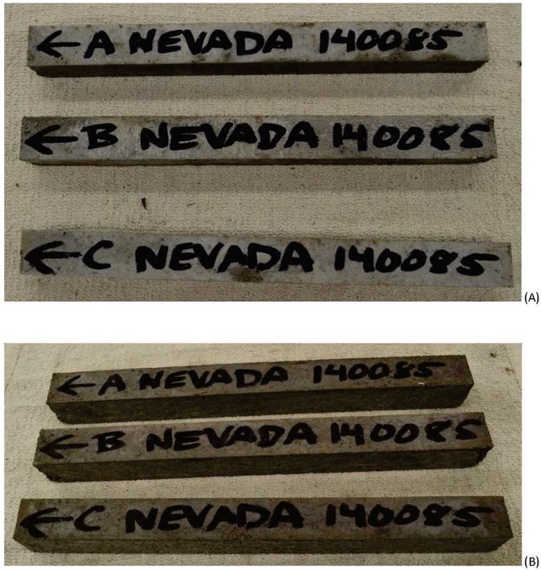
Figure A-13: Nevada Test Site 140085 (A) before autoclaving and (B) after autoclaving
