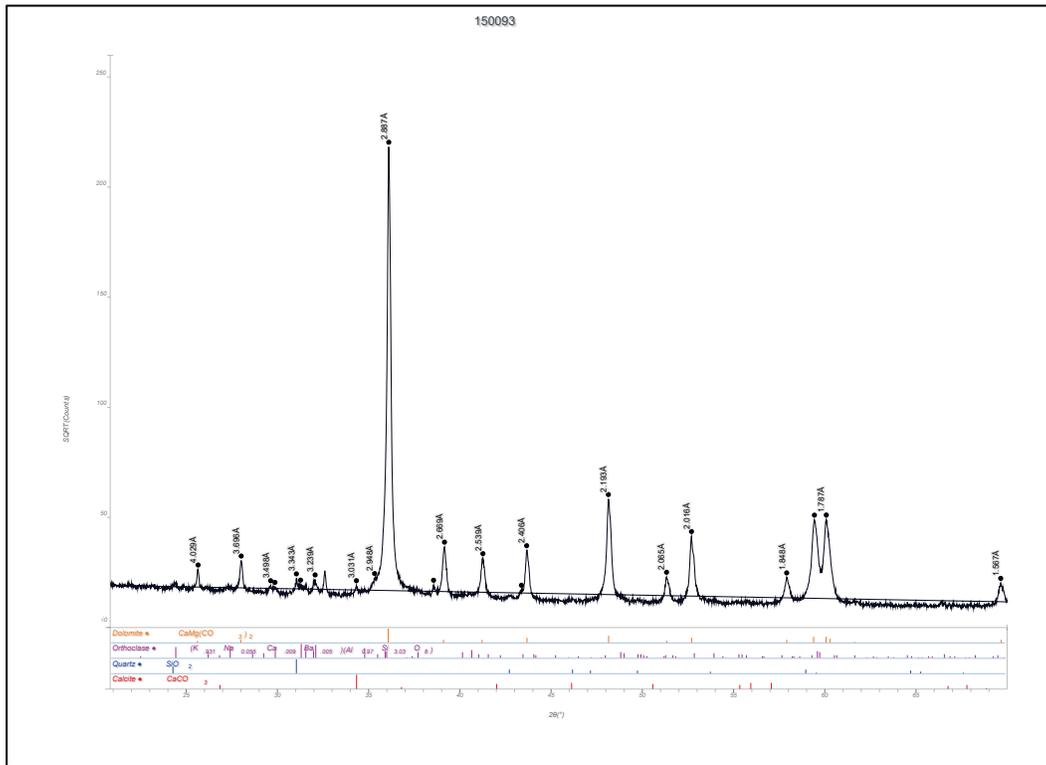
Figure B66. Whole pattern fit with mineral percentages Adairsville, Atlanta, GA, Fine Aggregate Sample (CMB No. 150093).
