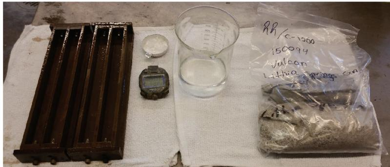
Figure 1. Sample Molds and As-Received Aggregates and Cement Materials for the Project
