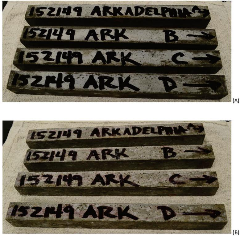
Figure A-16: Arkadelphia 152149 (A) before autoclaving and (B) after autoclaving
