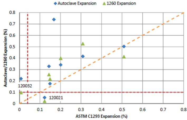
FIGURE 5: AUTOCLAVE AND ASTM C1260 EXPANSION RESULTS COMPARED TO ASTM C1293 EXPANSION
