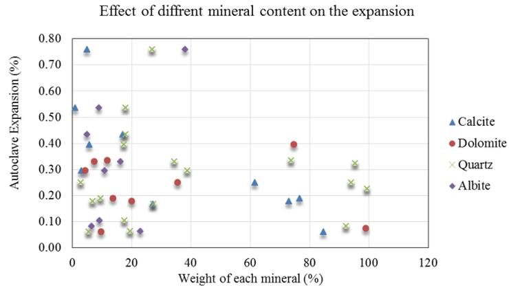
Figure 12. Correlation between selected mineral and the Autoclave expansion of mortar bars
