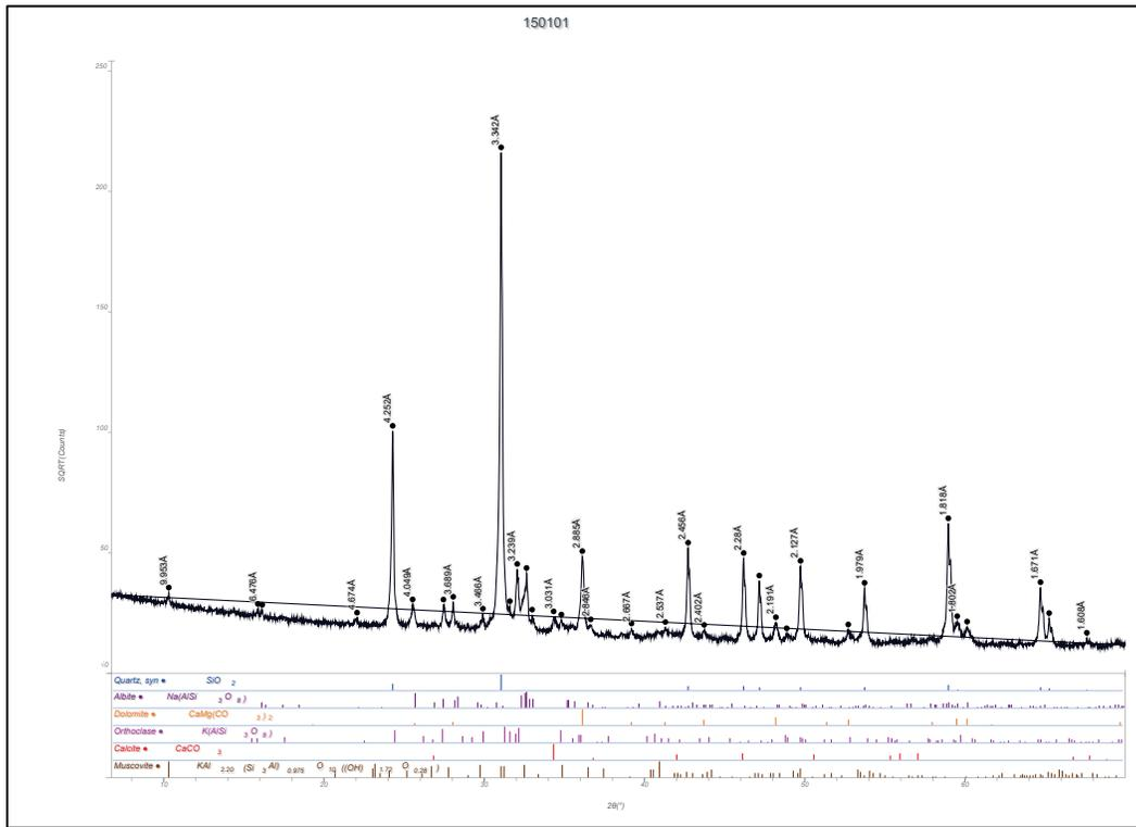
Figure B93. Whole pattern fit with mineral percentages Geneva, Utah, Fine Aggregate Sample (CMB No. 1500101).
