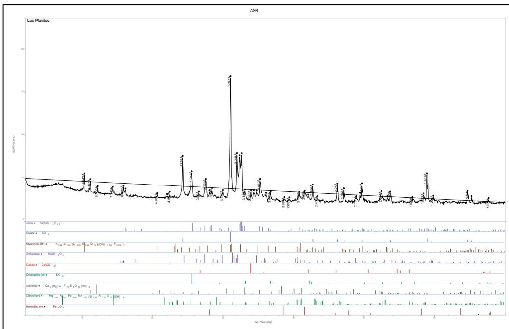
Figure B24. Whole pattern fit with mineral percentages Las Placitas Coarse Aggregate Sample (CMB No. 130006).
