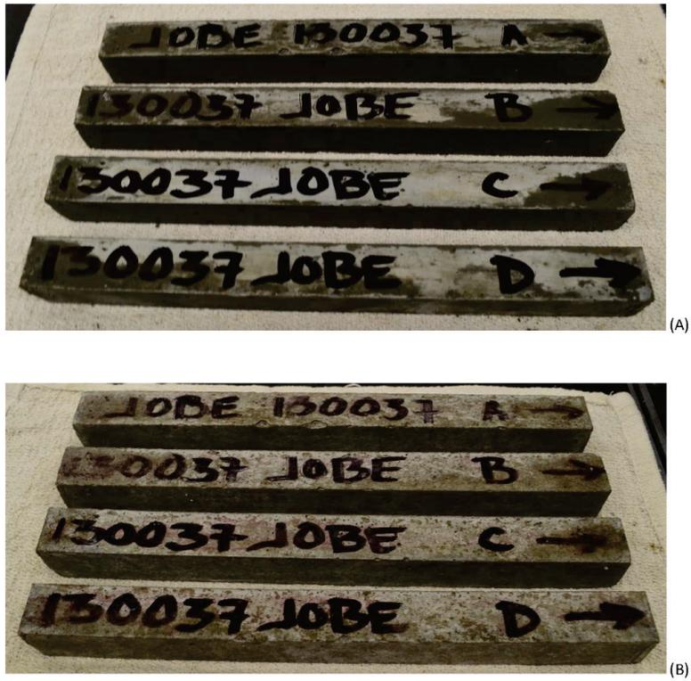
Figure A-15: Job 130037 (A) before autoclaving and (B) after autoclaving
