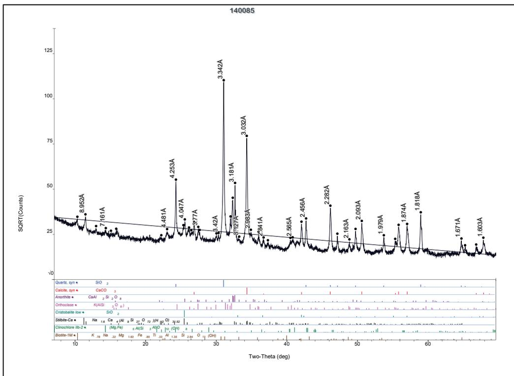
Figure B57. Whole pattern fit with mineral percentages Nevada Fine Aggregate Sample (CMB No. 140085).
