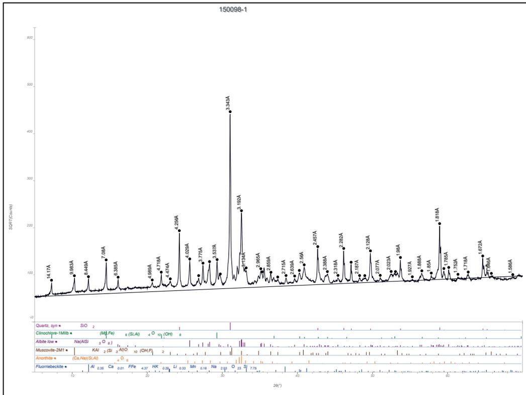
Figure B84. Whole pattern fit with mineral percentages Sudbury-Canada Coarse Aggregate Sample (CMB No. 150098.1).
