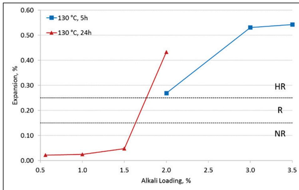
Although alkali leaching was not measured in this study, mortar bars with aggregate HR3 and alkali boosting up to 1.5% may have leached alkalis, resulting in insufficient alkalis in the mortar bars to promote ASR. A previous study by the authors showed alkali leaching between 4 and 11% for autoclaved concrete prisms (Wood et al. 2016).
