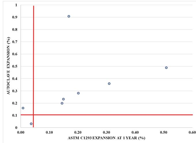
Figure 2: Comparison between ASTM C1293 and Autoclave Expansions
