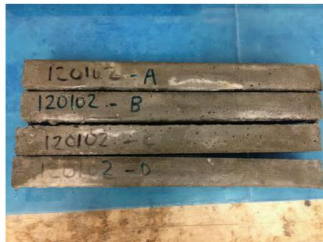
Aggregate 120102 Post Autoclave
