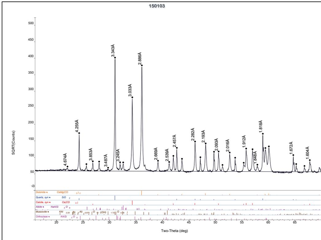
Figure B99. Whole pattern fit with mineral percentages Geneva, Utah, Coarse Aggregate Sample (CMB No. 150103).
