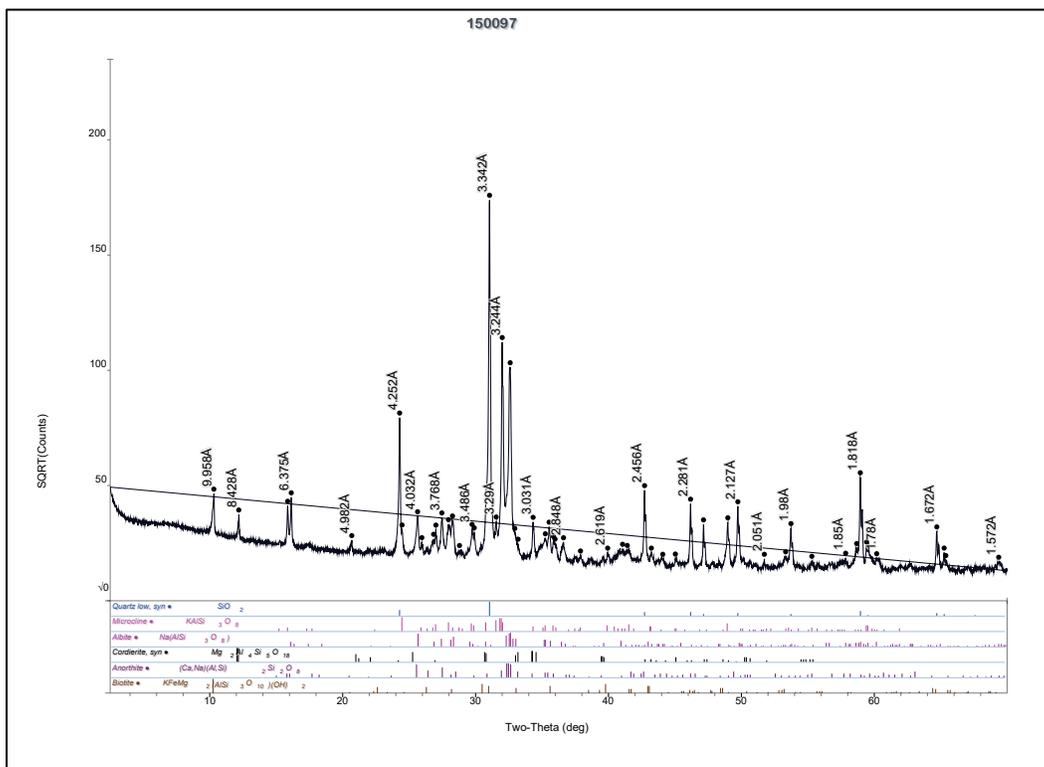
Figure B78. Whole pattern fit with mineral percentages Knife River, Cheyenne, WY, Fine Aggregate Sample (CMB No. 150097).
