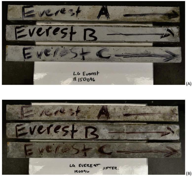
Figure A-17: LG Everist 150096 (A) before autoclaving and (B) after autoclaving
