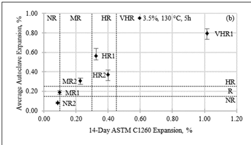
Figure 3. Autoclave expansions versus 14-Day ASTM C1260 expansions. Alkali loading, autoclaving temperature, and autoclaving duration were (a) 3.5%, 130 °C, and 24 hr and (b) 4.5%, 130 °C, and 5 hr.
