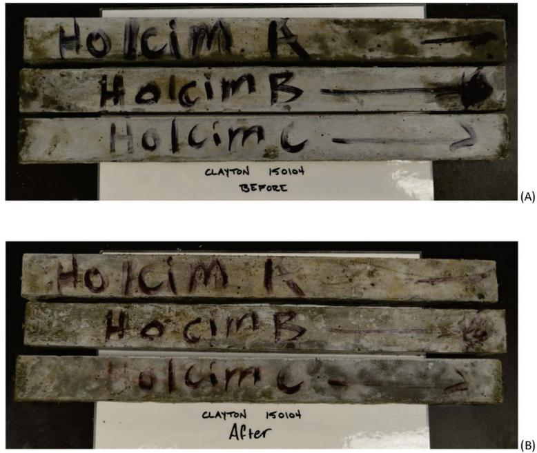
Figure A-8: Clayton 150104 (A) before autoclaving and (B) after autoclaving
