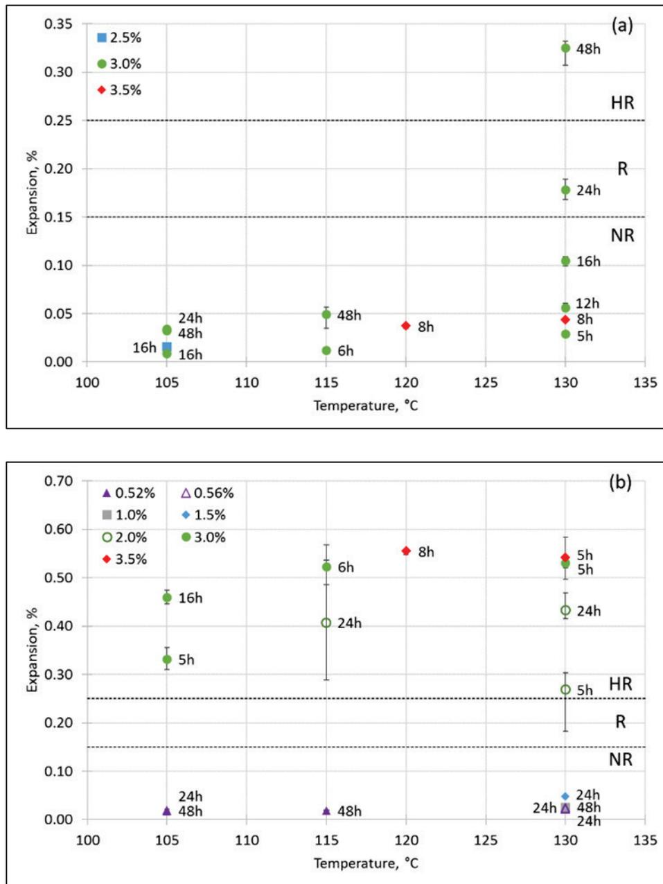
The highest average mortar bar expansion observed for aggregate NR1 (0.325%) occurred at 130°C with 3.0% Na<sub>2</sub>O<sub>eq</sub> conditioned for 48 hr. This was one of only two instances in which NR1 reached levels of expansion exceeding the proposed threshold for reactive aggregates in this study; it also appeared to be reactive when tested at 130°C using 3.0% Na<sub>2</sub>O<sub>eq</sub> for 24 hr.
