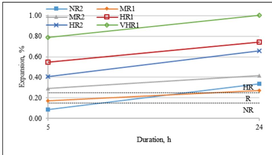
A summary of the changes in expansion resulting from modifications of the test parameters are provided in Table 4. The parameters in bold were altered while the other parameters listed were held constant. For instance, in the second column of the table, the differences in expansion are shown for an increase in alkali loading from 2.5 to 3.5% at 130°C for 5 hr; the factor is the expansion at 3.5% alkali loading divided by the expansion at 2.5% alkali loading.
