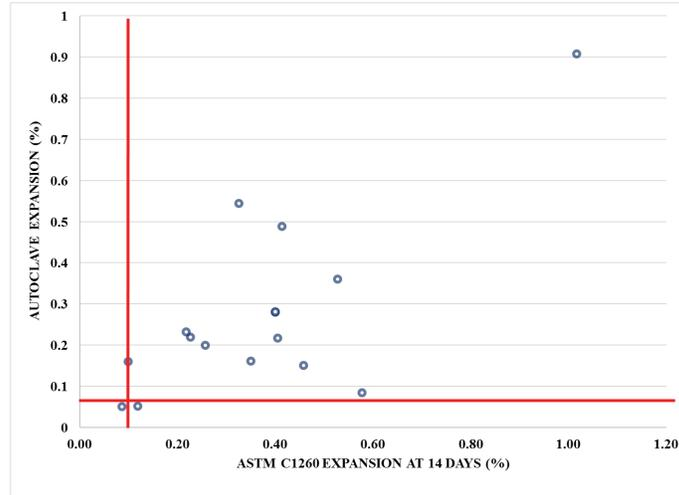
Figure 1: Comparison between ASTM C1260 and Autoclave Expansions
