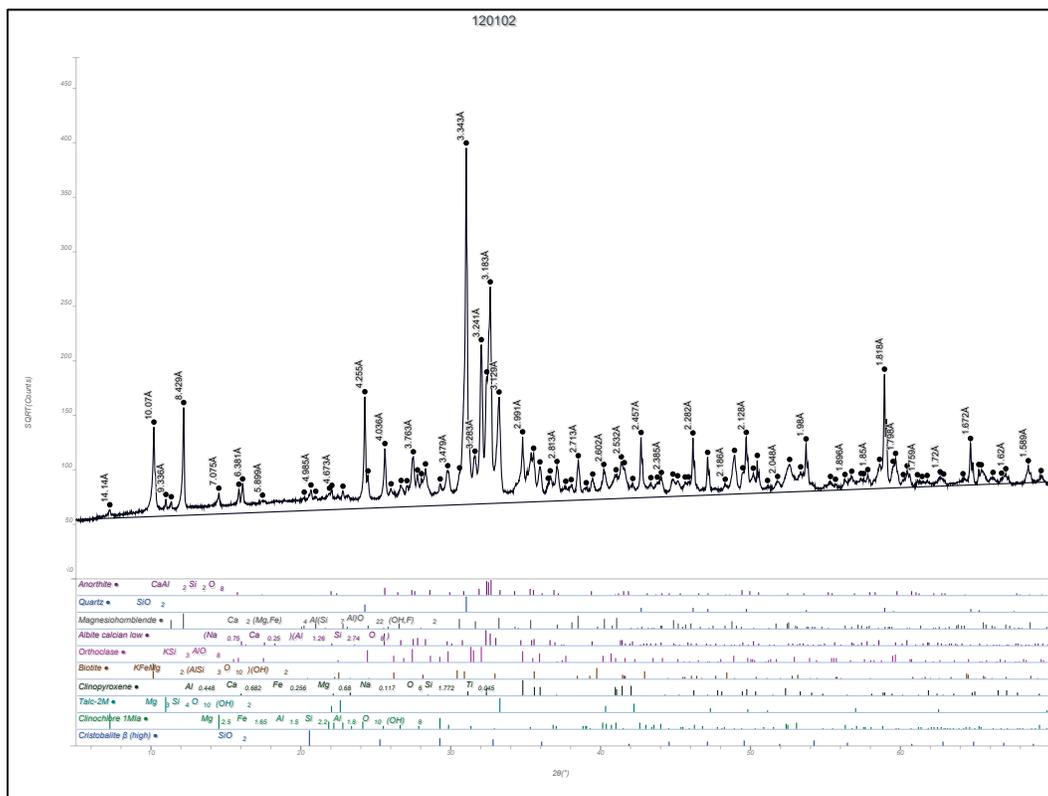
Figure B15. Whole pattern fit with mineral percentages China Lake Coarse Aggregate Sample (CMB No. 120102).
