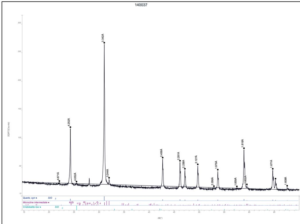
Figure B51. Whole pattern fit with mineral percentages Green Brothers Fine Aggregate Sample (CMB No. 140037).
