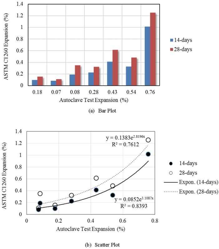
Figure 11. Correlation between expansion results from AMBT (14-days and 28-days) and Autoclave tests
