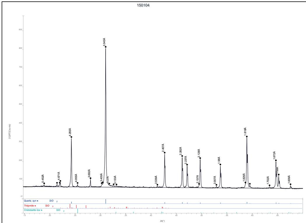
Figure B102. Whole pattern fit with mineral percentages Clayton/Yardville Fine Aggregate Sample (CMB No. 150104).
