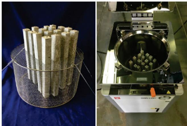
FIGURE 2: (LEFT) STAND FOR HOLDING THE SAMPLES AND (RIGHT) AUTOCLAVE AND MORTAR SAMPLES IN SITU
