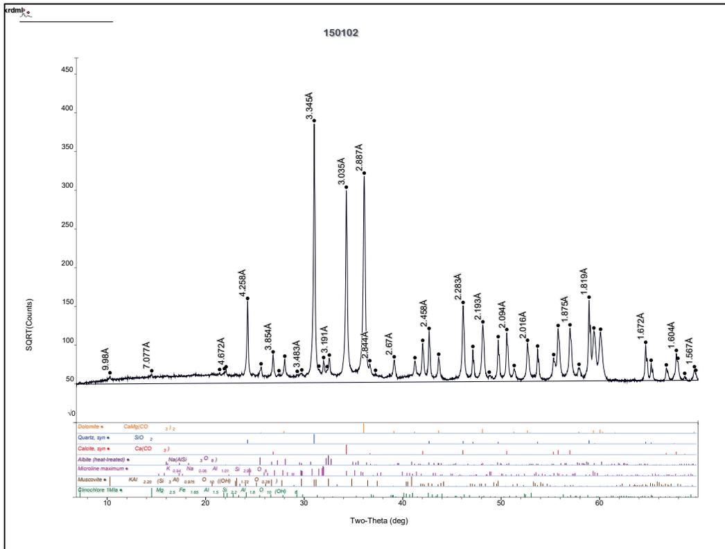
Figure B96. Whole pattern fit with mineral percentages Geneva, Utah, Fine Aggregate Sample (CMB No. 150102).
