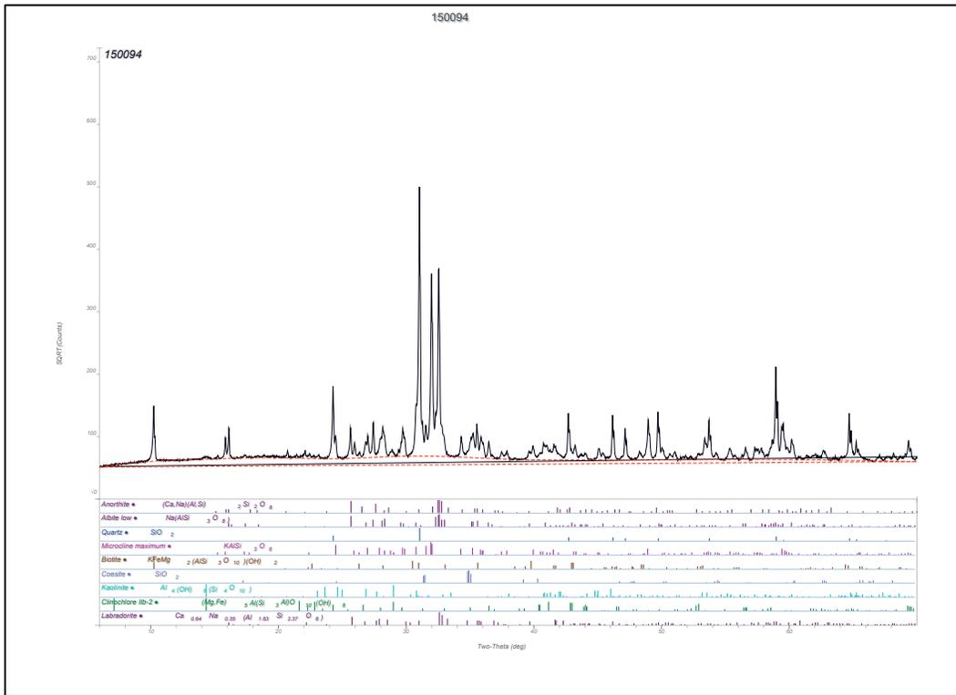
Figure B69. Whole pattern fit with mineral percentages Vulcan, Atlanta, GA, Fine Aggregate Sample (CMB No. 150094).
