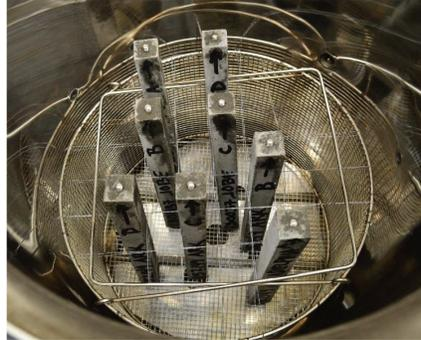
Figure 3-2: Mortar bars positioned upright inside the autoclave.
