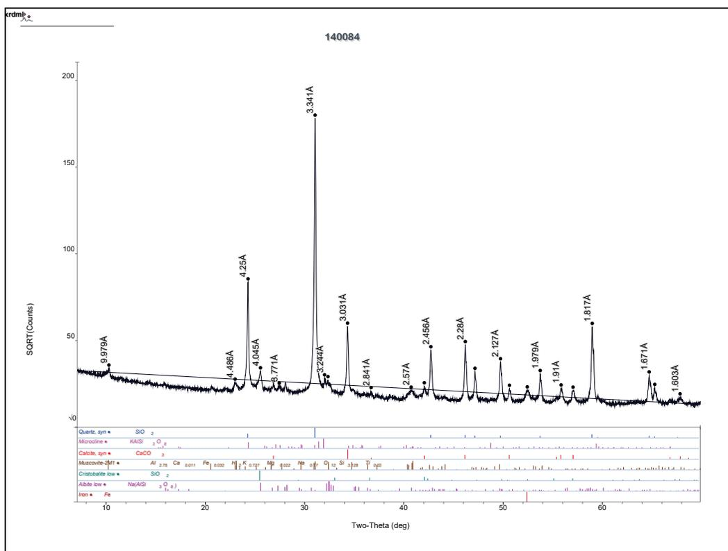
Figure B54. Whole pattern fit with mineral percentages Nevada Coarse Aggregate Sample (CMB No. 140084).
