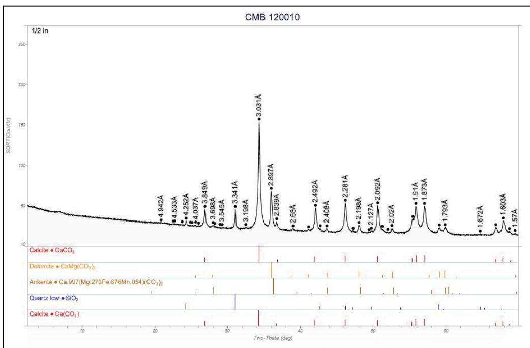
Figure B3. Whole pattern fit with mineral percentages for Vulcan-Cookeville Coarse Aggregate Sample (CMB 120010).
