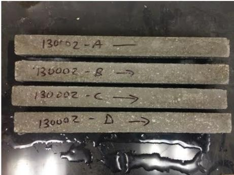
Aggregate 13002 Post Autoclave
