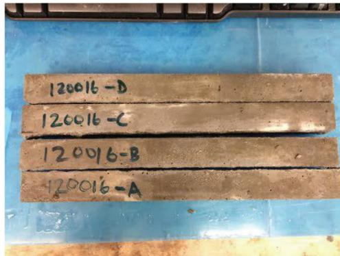
Aggregate 120016 Post Autoclave
