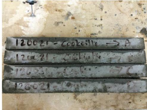
Aggregate 120021 Post Autoclave
