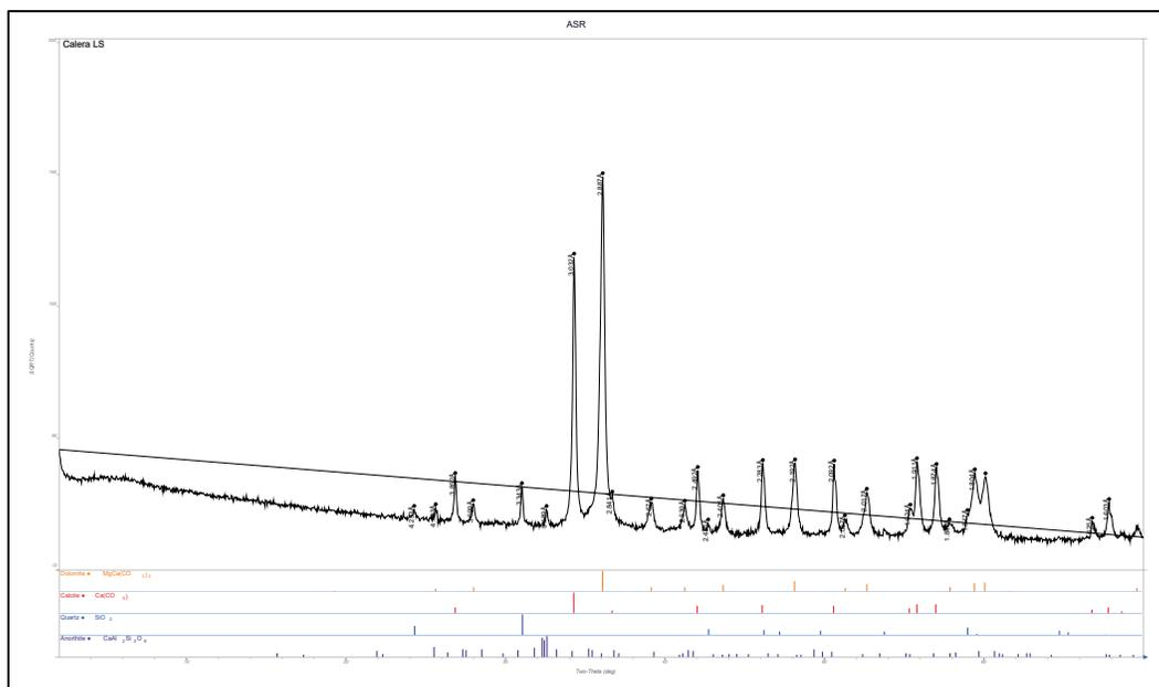
**Figure B39. Whole pattern fit with mineral percentages Calera Coarse Aggregate Sample (CMB No. 130040).**
