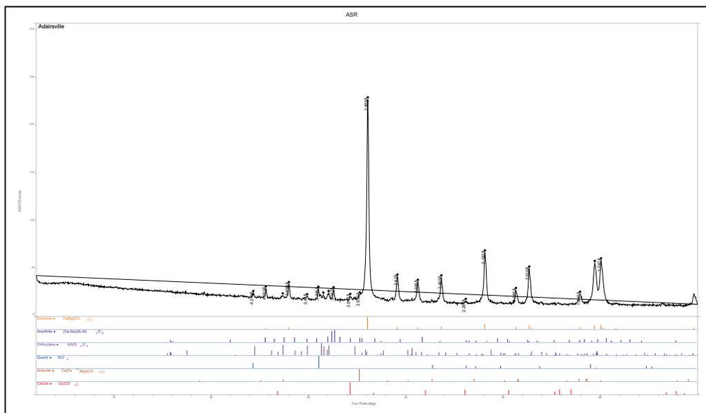
Figure B33. Whole pattern fit with mineral percentages Adairsville Coarse Aggregate Sample (CMB No. 130038).
