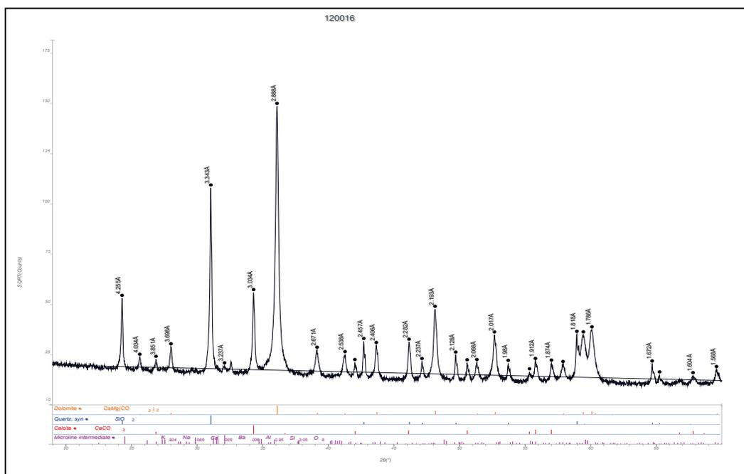
Figure B6. Whole pattern fit with mineral percentages Rogers-Gordonville Coarse Aggregate Sample (CMB No. 120016).
