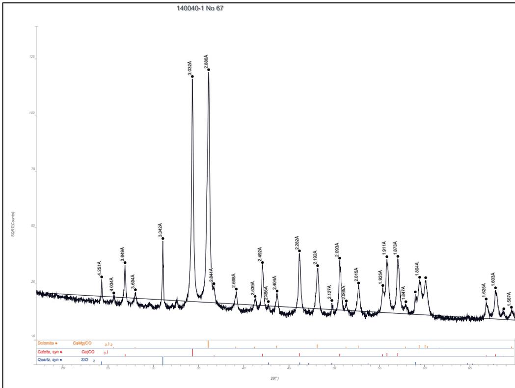
Figure B45. Whole pattern fit with mineral percentages Calera Coarse Aggregate Sample (CMB No. 130040 - No. 67).
