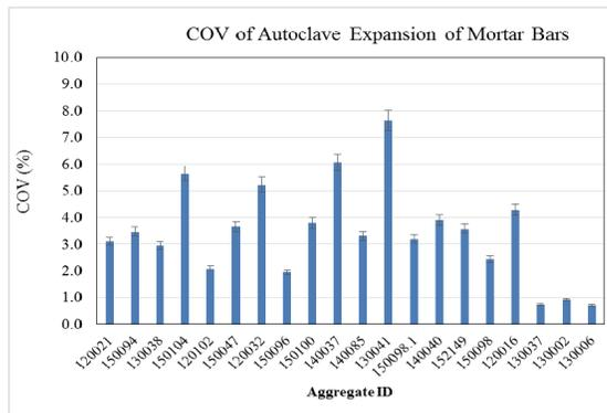
Figure 5. COV of autoclave expansion results of mortar bars made with different type of aggregates
