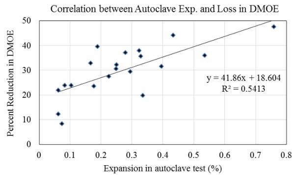
Figure 10. Correlation Between Autoclave Expansion and Loss in Dynamic Modulus of Elasticity
