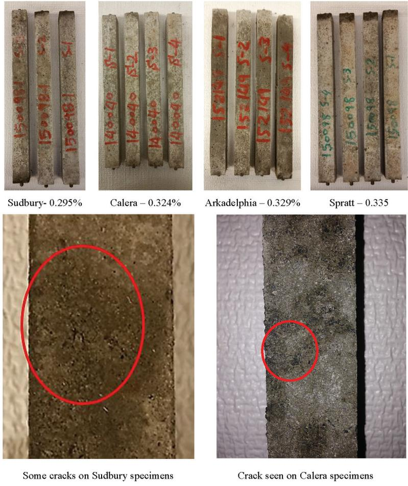
Figure 8. Photographs of Mortar Bars Subjected to Autoclave Testing (exp > 0.29% & < 0.40)
