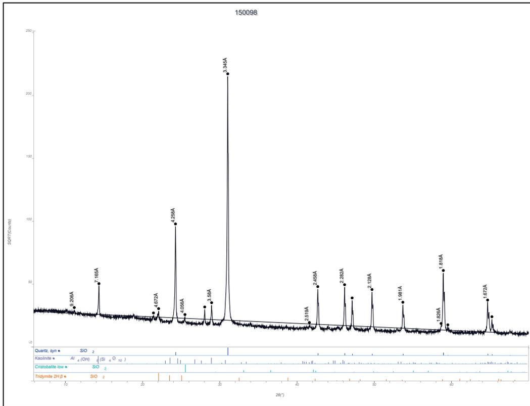
Figure B75. Whole pattern fit with mineral percentages LG Everist Dell Rapids, SD, Fine Aggregate Sample (CMB No. 150096).
