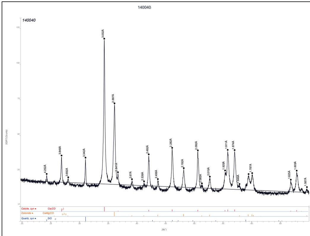
Figure B48. Whole pattern fit with mineral percentages Calera Coarse Aggregate Sample (CMB No. 130040).
