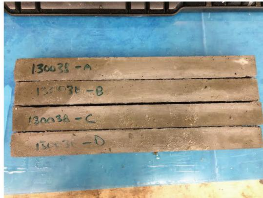
Aggregate 130038 Post Autoclave
