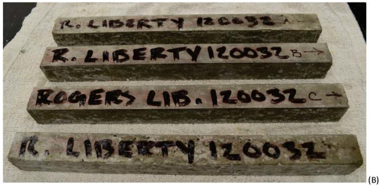
Figure A-4: Rogers Liberty 120032 (A) before autoclaving and (B) after autoclaving
