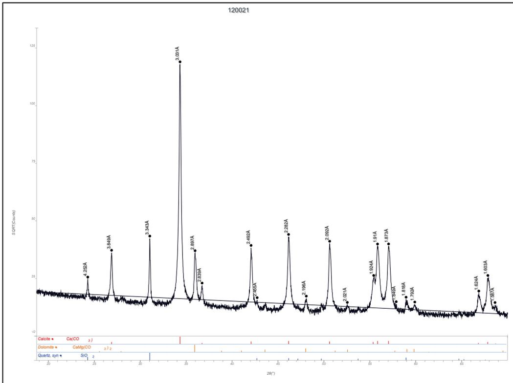
Figure B9. Whole pattern fit with mineral percentages Cookville Coarse Aggregate Sample (CMB No. 120021).
