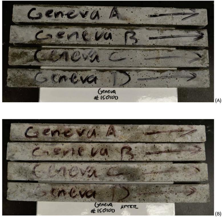
Figure A-18: Geneva 150100 (A) before autoclaving and (B) after autoclaving
