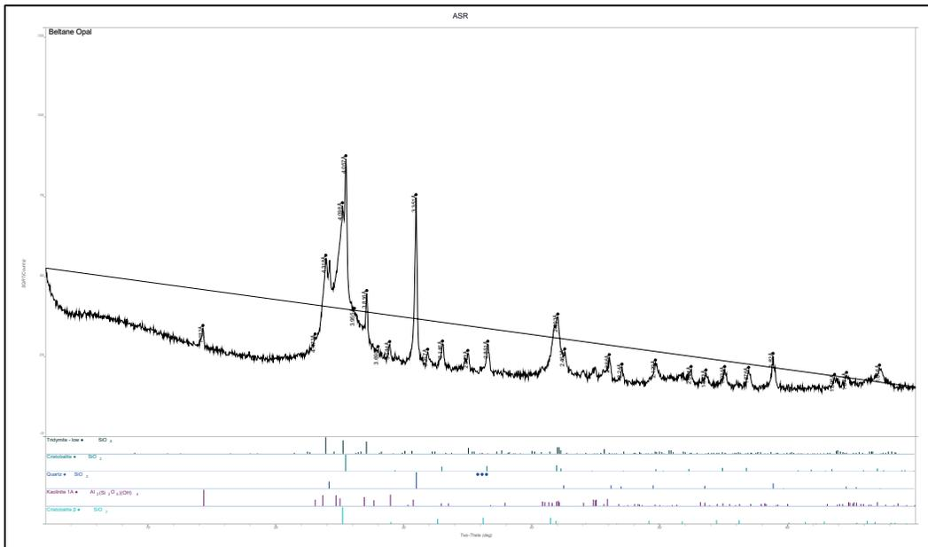
Figure B36. Whole pattern fit with mineral percentages Beltane Opal Coarse Aggregate Sample (CMB No. 130039).
