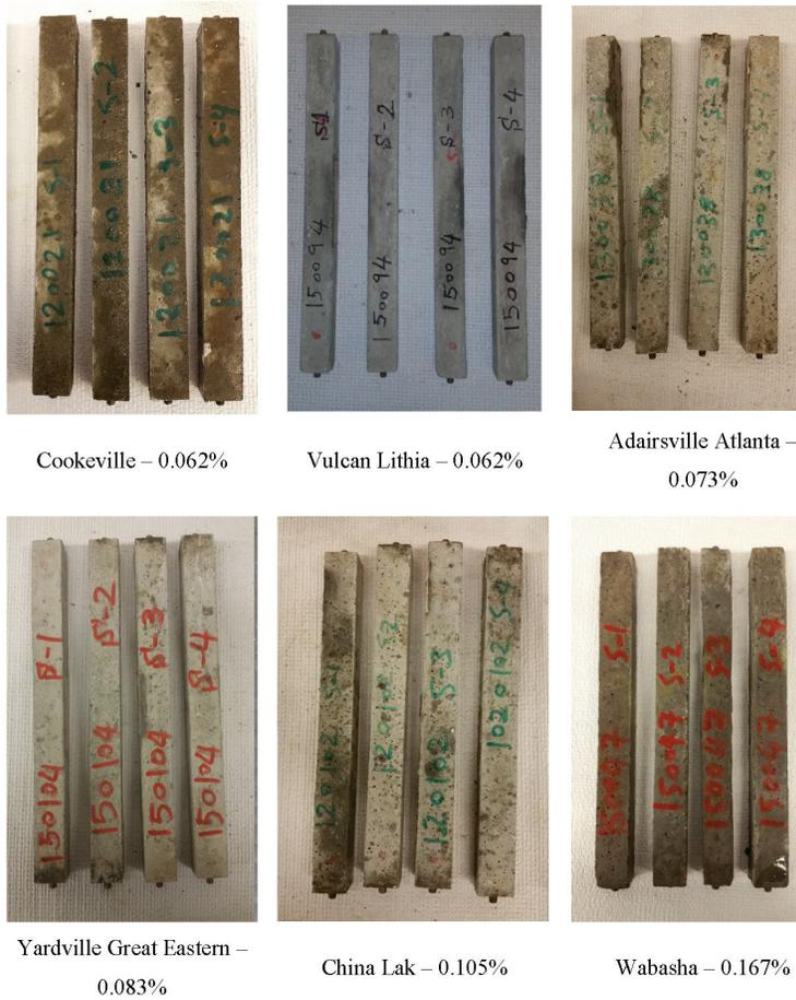
Figure 6 – Photographs of Mortar Bars Subjected to Autoclave Test (exp < 0.28%)
