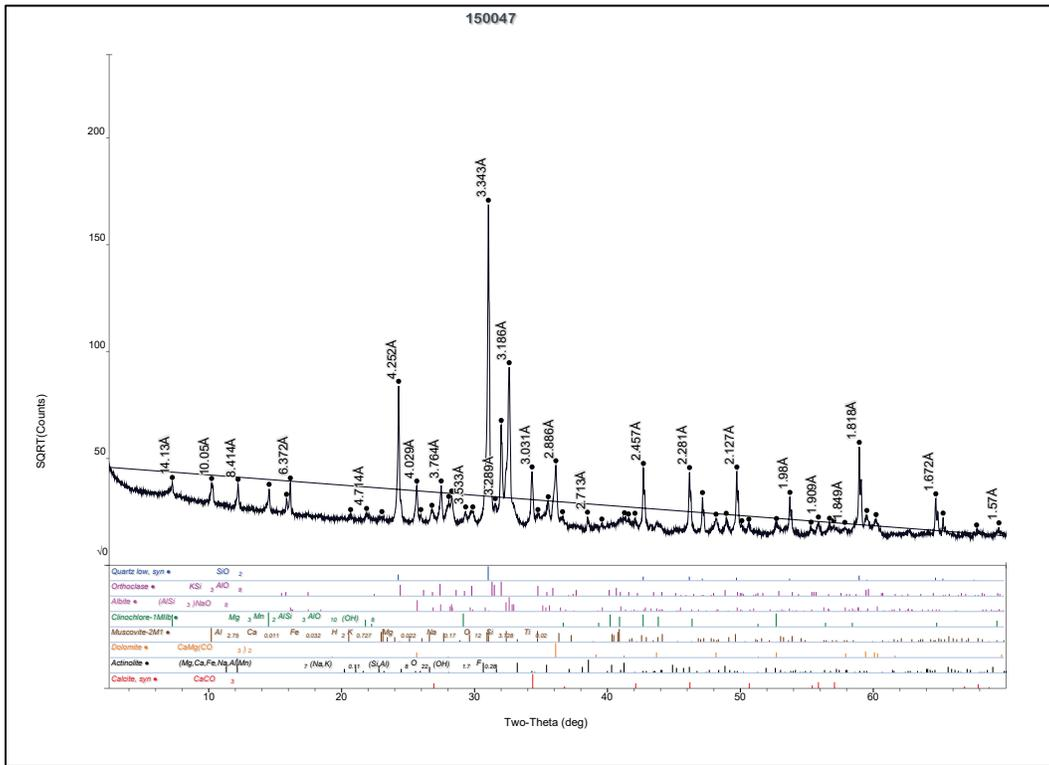
Figure B63. Whole pattern fit with mineral percentages Wabasha, MN, Fine Aggregate Sample (CMB No. 150047).
