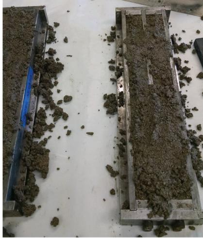
Figure 4-1: Nevada Test Site (140085) mixture crumbling during placement.
