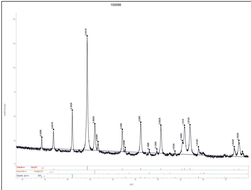
Figure B81. Whole pattern fit with mineral percentages Spratt-Canada Coarse Aggregate Sample (CMB No. 150098).
