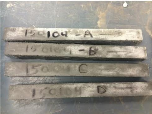
Aggregate 150104 Post Autoclave
