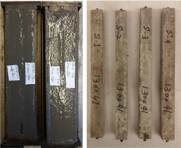
Figure 2. Specimens just after the molding (left), and specimens after 48 h of curing (right)
