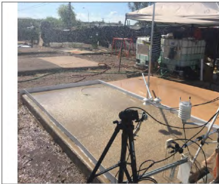
Figure 3. Heavy artificial rain generated over the impervious concrete surface
