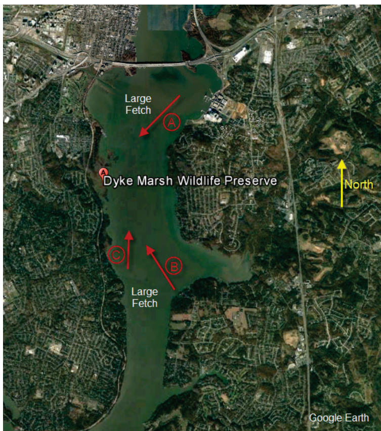
Figure 5-2. Map of the Dyke Marsh area. Arrows indicate directions from which winds blowing would have the potential to create larger wind-waves due to larger fetches.
