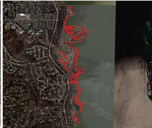
Figure 4-8. Topo-bathymetric data points surveyed in 2009, 2012, and 2016.
