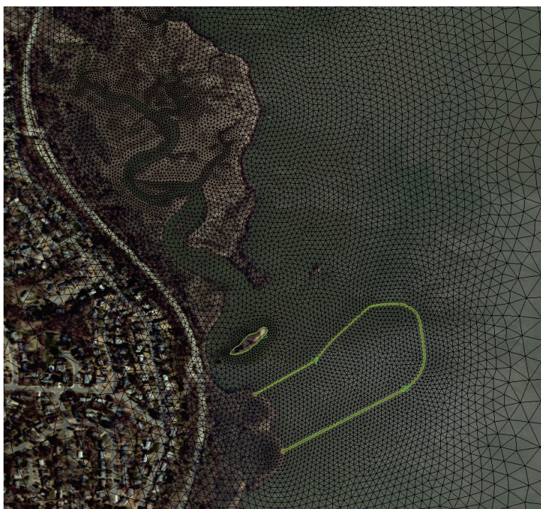
Figure 5-7. Refined computational grid (20 ft resolution in the Dyke Marsh).
