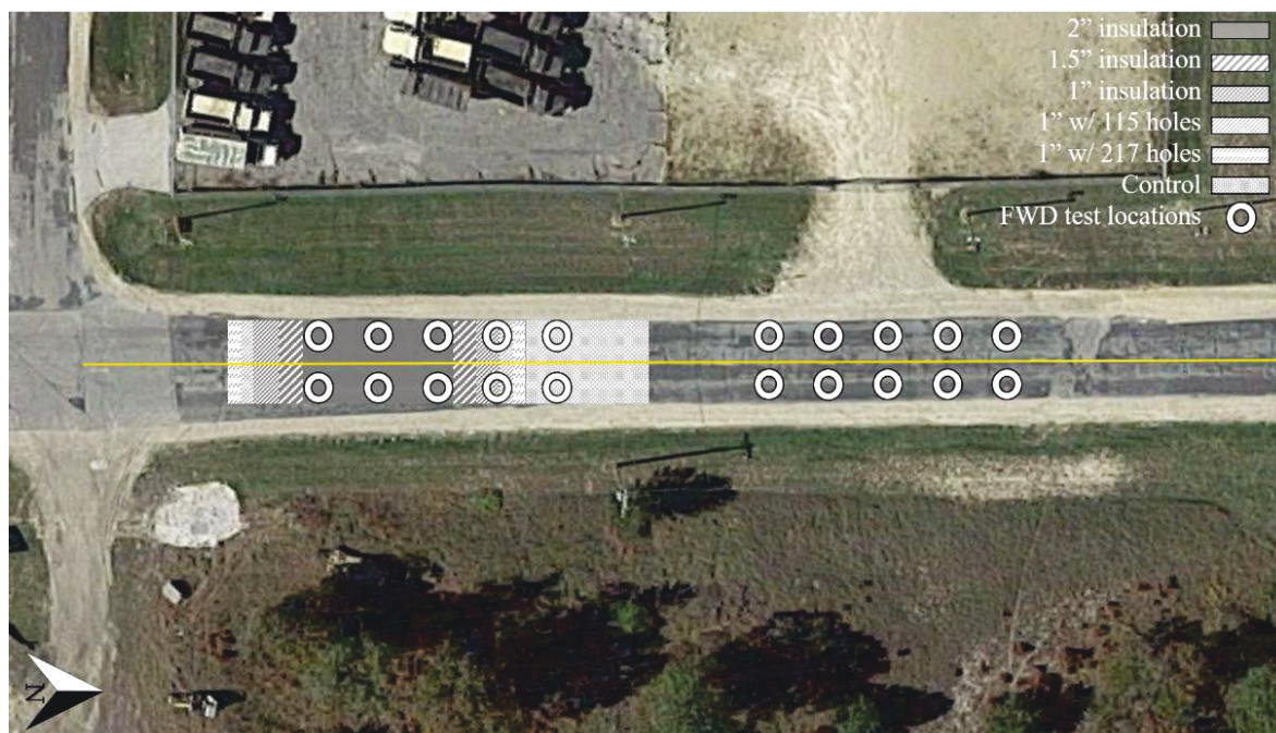
Figure 3. Approximate locations of the falling weight deflectometer (FWD) tests performed on East South Street at Fort McCoy.
