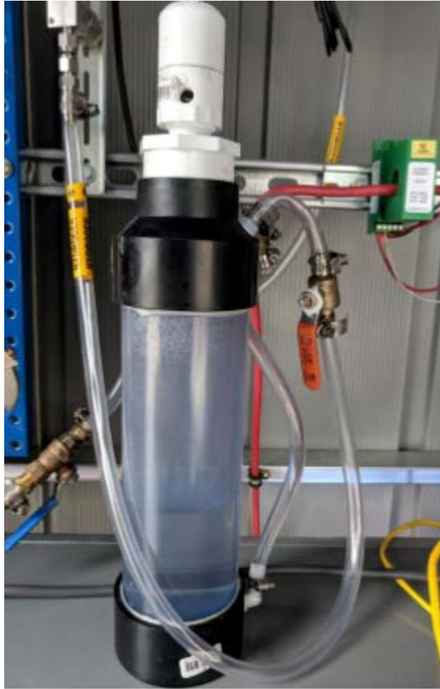
Figure 10. Bubbler for Humidification of the Hydrogen Working Fluid with a Low-Pressure Release Valve
