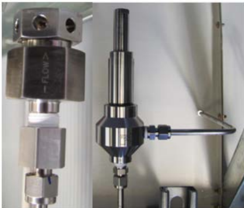
Figure 11. Rupture Disc (left) and Proportional Relief Valve (right) Overpressure Safety Systems
