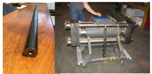
7.62 mm barrel for external pressure rifling with electric opening pressure chamber
