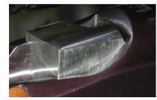
Drop Block (Tapered?) Interrupted Helical Lug
