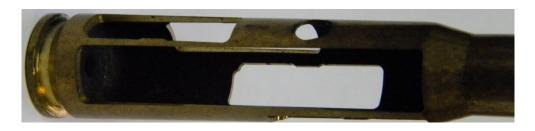
Micro Hardness Sample from Case Sidewall
