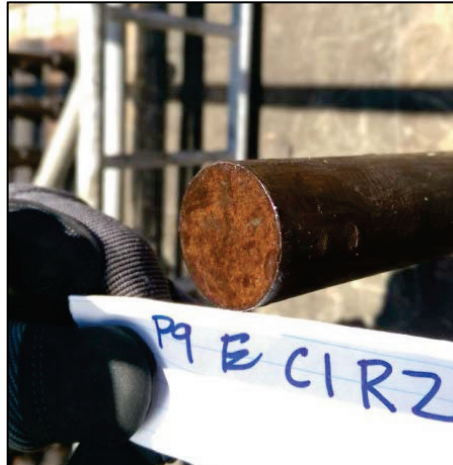
Figure 5. Typical rod without corrosion.
