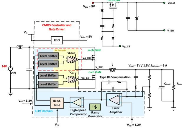
Fig. 2. Detailed block diagram of the presented hybrid CMOS/GaN buck converter.
