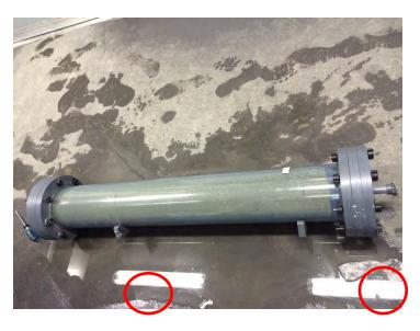
Figure 1-Zeolite Column; circled in red are the pieces that sit into the equipment skid, which made alignment and support of the column possible.
