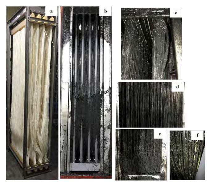
Figure 5.54 GAC-fluidized AnMBR Ultrafiltration Membrane Modules Prior to (a) and After (b) the Demonstration. Close-up Photos of the Top (c), Middle (d), and Bottom (e,f) of the Fibers After (d,f,h) the Demonstration.
