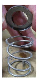
A small hook may be needed to remove the lower part of the mechanical seal. Be **EXTREMELY** careful when using a tool to remove the mechanical seal. If the ceramic part of the seal breaks, the entire assembly will need to be replaced.
