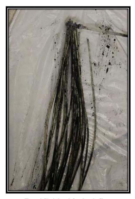
Figure 6: Black deposit found on the fibers.
