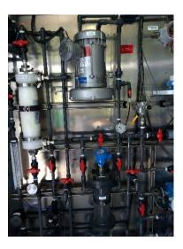
Figure 3 - Hollow fiber membrane with respect to the vacuum pump and the condensate trap.
