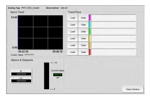
This screen will allow the user to set any high or low alarm limits associated with the instrument, as well as view a "quick-trend" of its recent activity. To add this analog signal to the main trending screen, simply press "Load" on one of the open Trend Pens.
