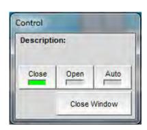
controlled by the sequencer (activated from the Overview Screen). Pressing the CLOSE or OPEN control buttons will actuate the valve independent of the sequencer.
