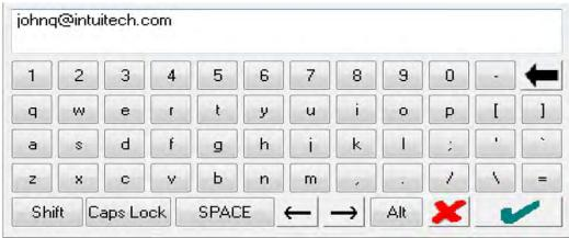
The full keypad is displayed anytime alpha-numeric characters are required. Each keypad is displayed when required.
