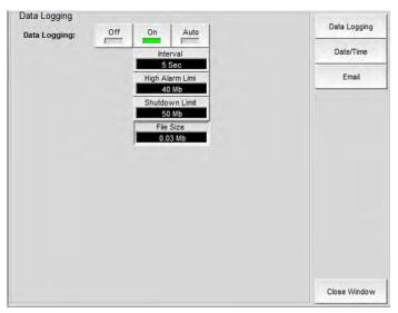
When in the automatic mode, the data-logging feature is only active when the system is active (i.e. data are only logged for equipment in operation).
