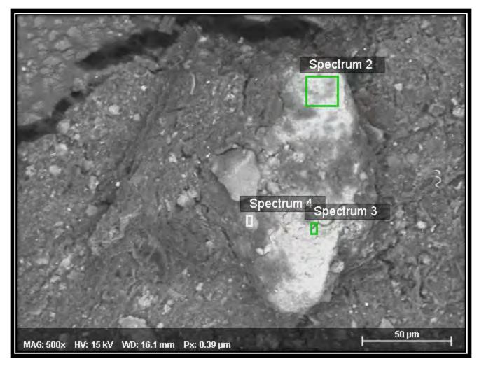
Figure 15: Electron micrograph of the membrane surface at 500X magnification (Spectrum 2, Spectrum 3 & Spectrum 4).
