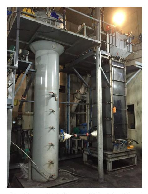
Figure 5.8 Photograph of the First-stage (AFBR - left) and Second-stage (AFMBR - right) GAC-fluidized AnMBR Systems.
