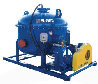
The vacuum degasser is used to remove the small entrained gas bubbles left in the mud by the mud/gas separator. These units are positioned downstream from mud/gas separators, gumbo removal equipments (if utilized), shale shakers, and mud conditioners (if utilized) while hydrocyclone desanders and decanting centrifuges follow in the arrangement.
