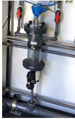
Figure 7 – Condensate Trap (Collection Tank)
