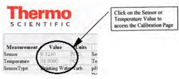
probe. To access the calibration screen, press the instrument configuration button. Once connected, the above screen will appear. To begin a calibration, simply click on the sensor value displayed, this will open the calibration screen. Then enter the value of the calibration standard and press "Set".
