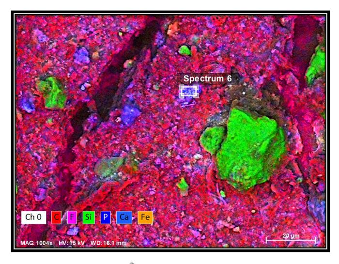
Figure 28: Superimposed Elemental Imaging (SEI®) of Organic based matter, silts/clays, phosphate salts (aluminum, calcium and iron), iron hydroxide, calcium sulfate and titanium oxide.
