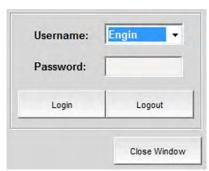
left corner of the screen. For security purposes, the passwords for each user level will not be printed in this manual. (Password information will be sent with the manual in a sealed envelope.) Select the LOGOUT button to return to the Guest level of access. Below are the five user levels and what functions each user has access to. Some activities may not be relevant for all HMI applications.
