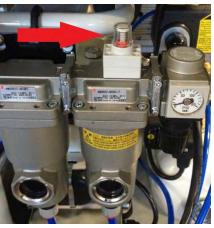
up and fills the clear window completely (red arrow) the filter element should be replaced.
