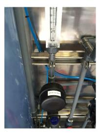
Figure 1 – The air filter that the ambient air will pass through before entering the membrane.
