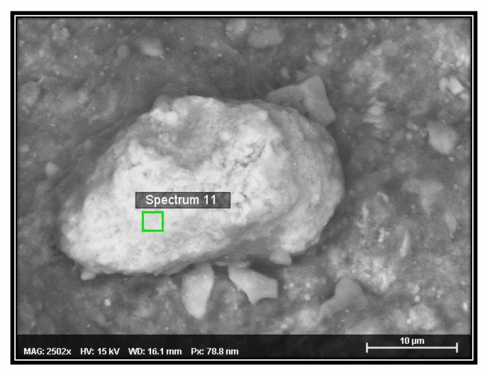
Figure 42: Electron micrograph of the membrane surface at 2500X magnification (Spectrum 11).
