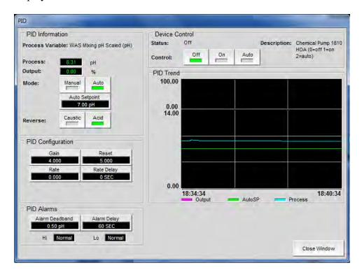
**NOTE:** All module components which operate using PID control (listed below) will be controlled by a screen very similar to this one.
