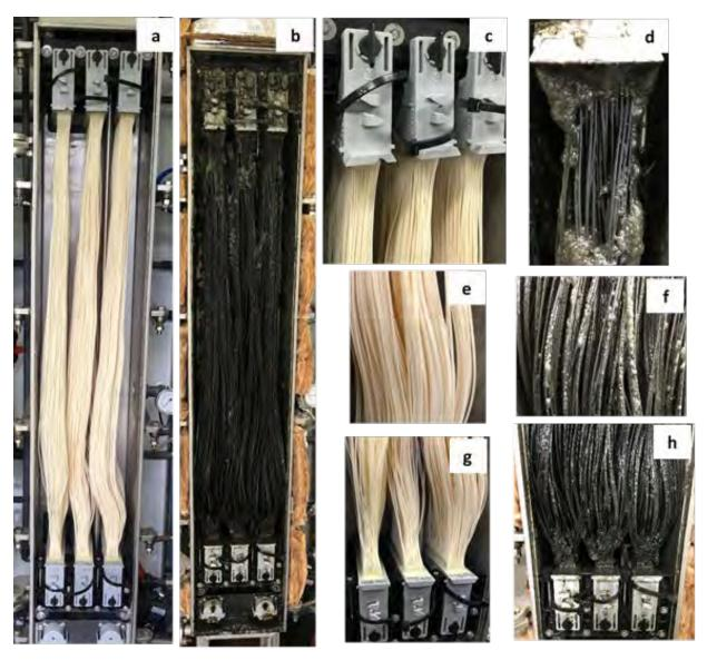
Figure 5.47 Gas-sparged AnMBR Ultrafiltration Membrane Modules Prior to (a) and After (b) the Demonstration.
