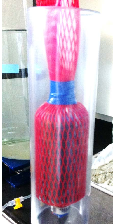
Figure 3-9. Laboratory tested passive flux meter.
