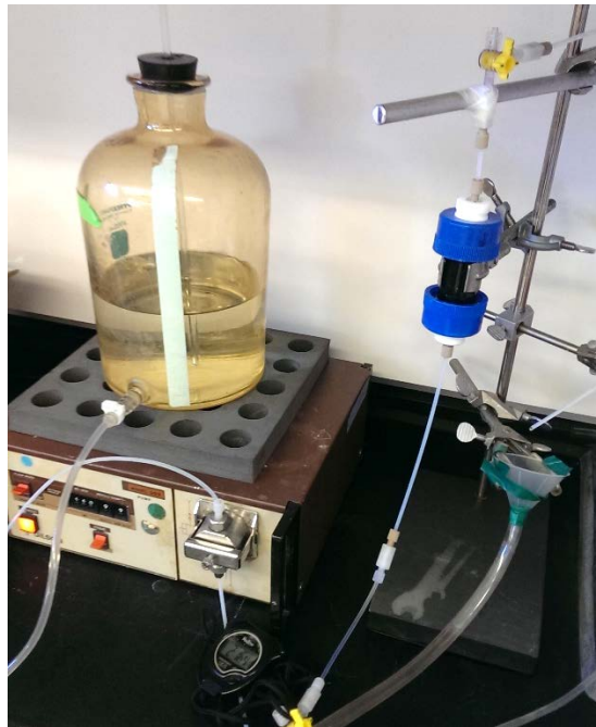
Figure 3-2. Column test setup.
