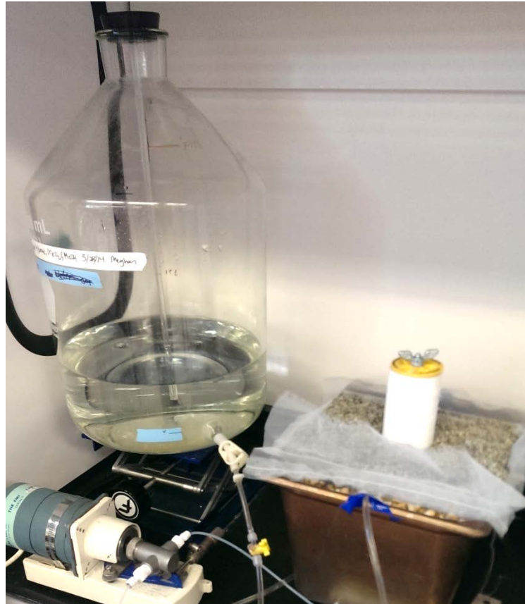
Figure 4-5. Box aquifer setup for extensive testing on the modified PFM design. Photo courtesy of Meghan Thiemann.
