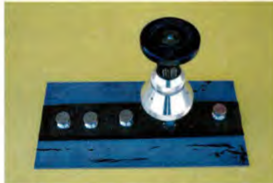
Coal tar urethane sample with 3/4" pull-off coupons and adherence tester.
