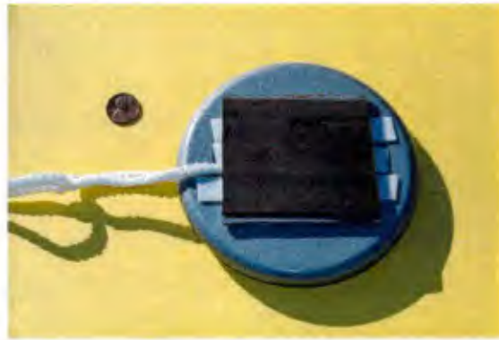
Coating sample attached to a 2.5 pound weight.
