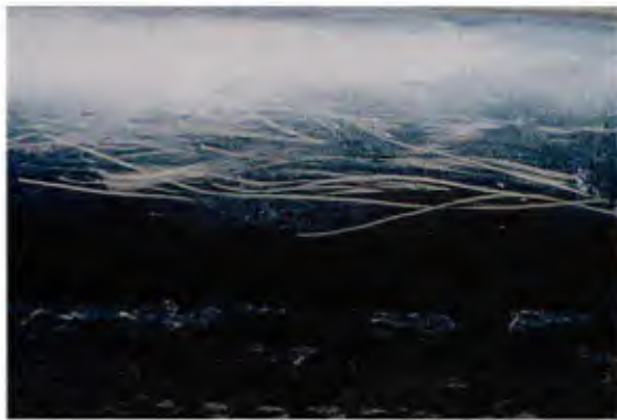
Light rubbing using shell embedded soil on coating: Sandpaper equivalent, 60 – 80 grit.
