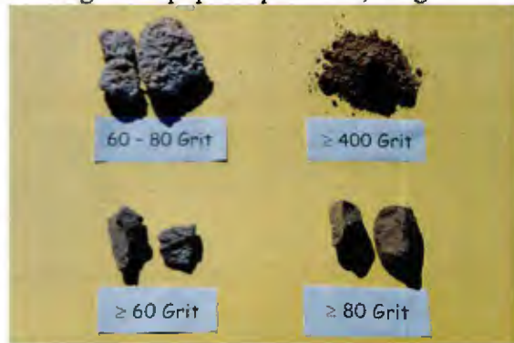
Top to Bottom (L to R): Shell embedded soil, soil, pumice type rock, and sand stone.
