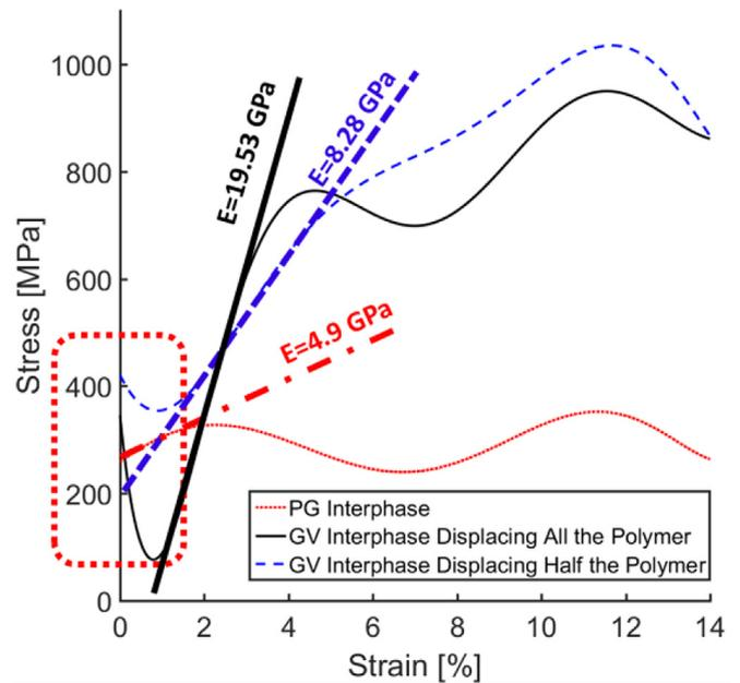
Fig. 9. Stress-strain plots from the virtual test results of the interphase models.
