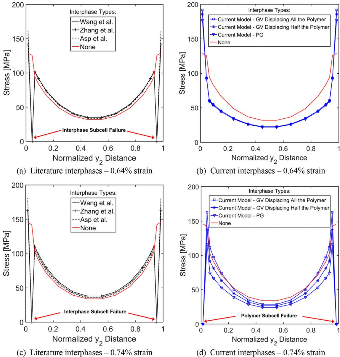
Fig. 12. Subcell stress-width plots for unit cell simulations.
