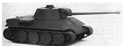
Figure 2. A wooden model of Daimler-Benz's recommended version for the Mark V Panther. The prototype was named VK3002 and had some clear similarities to the Soviet T-34 tank.
