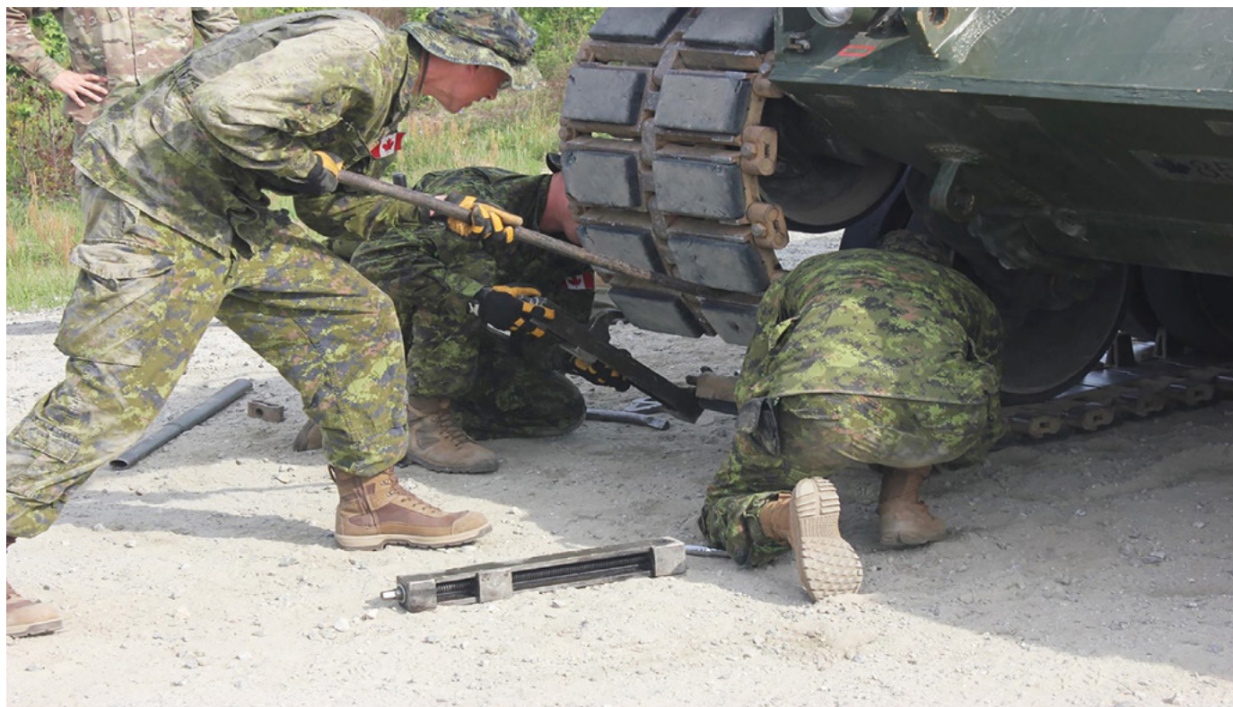
Figure 3. The Royal Canadian Armoured Corps Crew assembles tank track on the tank-maintenance lane during the situational-training exercise of the 2016 Sullivan Cup. (Photo by 194 th Armor Regiment Public Affairs)
