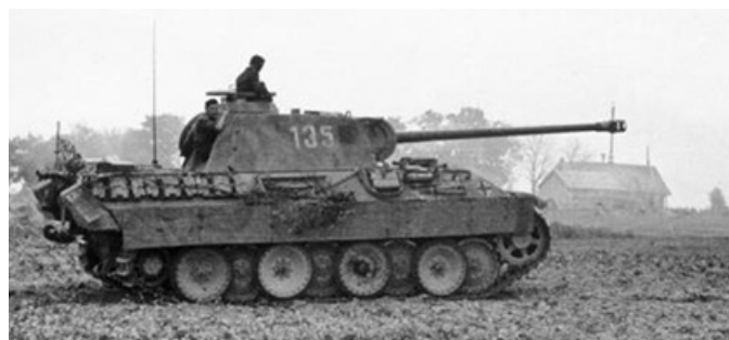
Figure 3. Panther with full Schürzen spaced armor attached, intended to supplement the side armor above the large wheels.
