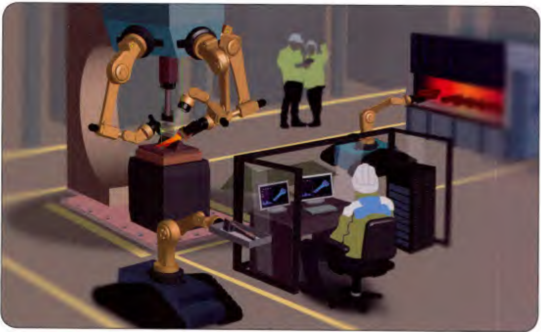
Figure 11. Conceptual metamorphic manufacturing equipment suite (containing the five fundamental elements of metamorphic manufacturing represented by the acronym STARC).
