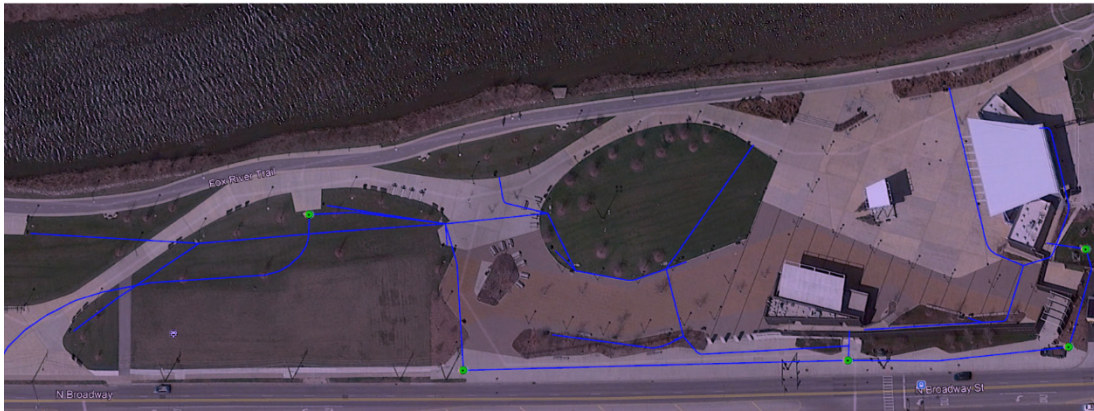
Figure 1. Fiber Optic Network at RiverEdge Park
