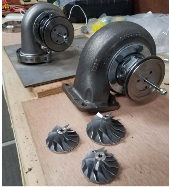
Figure 23. GT2554R (background) and GT3071R (foreground) with Compressor Wheels Removed
