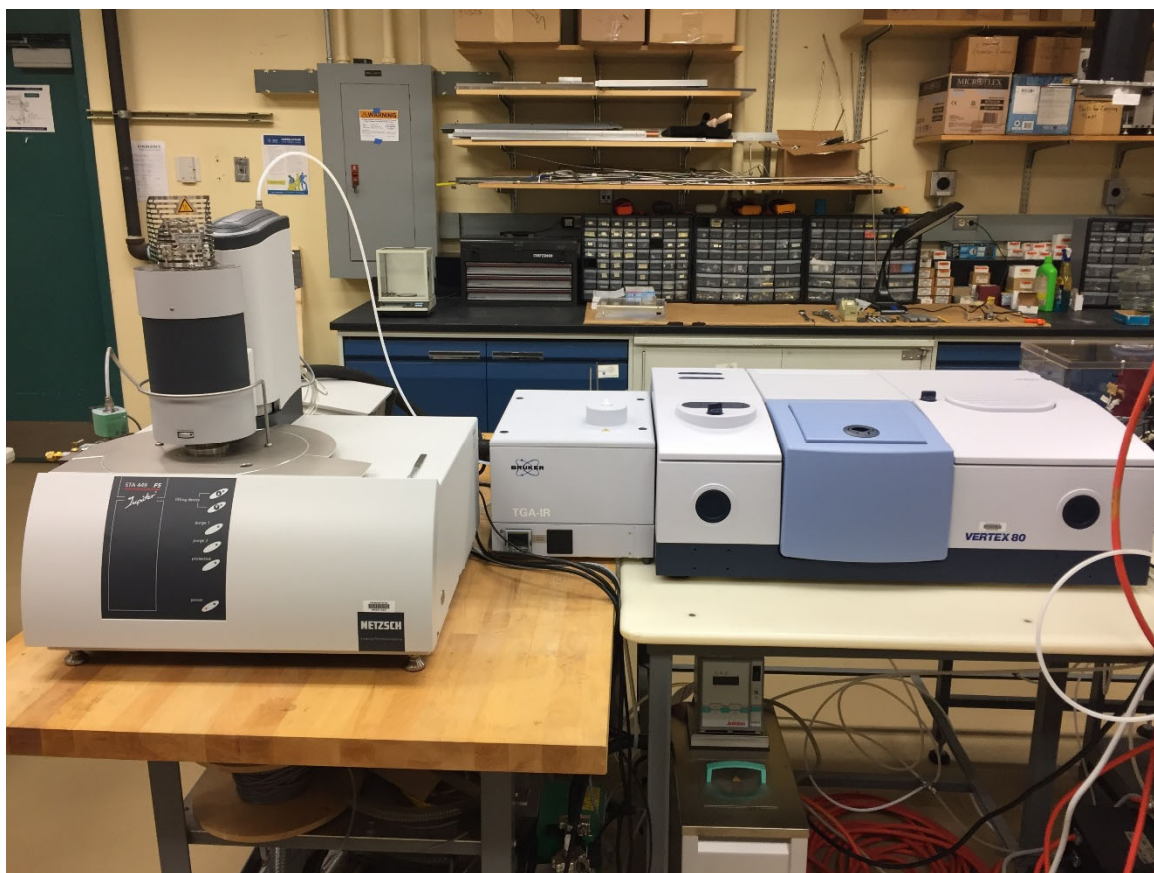
Figure 1. Components of the TGA/DSC/DTA interfaced to the Bruker Vertex 80 FTIR spectrometer are shown. The left component is the TGA, and the Vertex 80 is to the right. In the middle, attached to the Vertex 80, is the TGA interface. On the floor and not clearly shown are the chiller and the vacuum pump.
