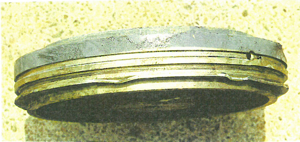
Figure 9. Rocket Motor Malfunction, Motor Nozzle View
