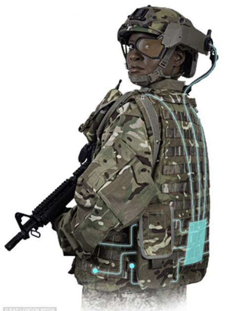
Figure 3-1: Power Distribution Through the Soldier Vest [50].
