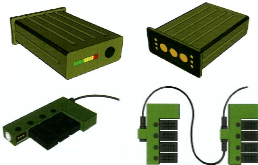
Figure 2-11: The Modular Rechargeable Battery of the Future Power Management System. These batteries have an energy content of 27 Wh (3 x 18650 Li-ion cells) and weigh 250 g. They have rotationally symmetric contact pins and communicate via SMBus to the system [17].
