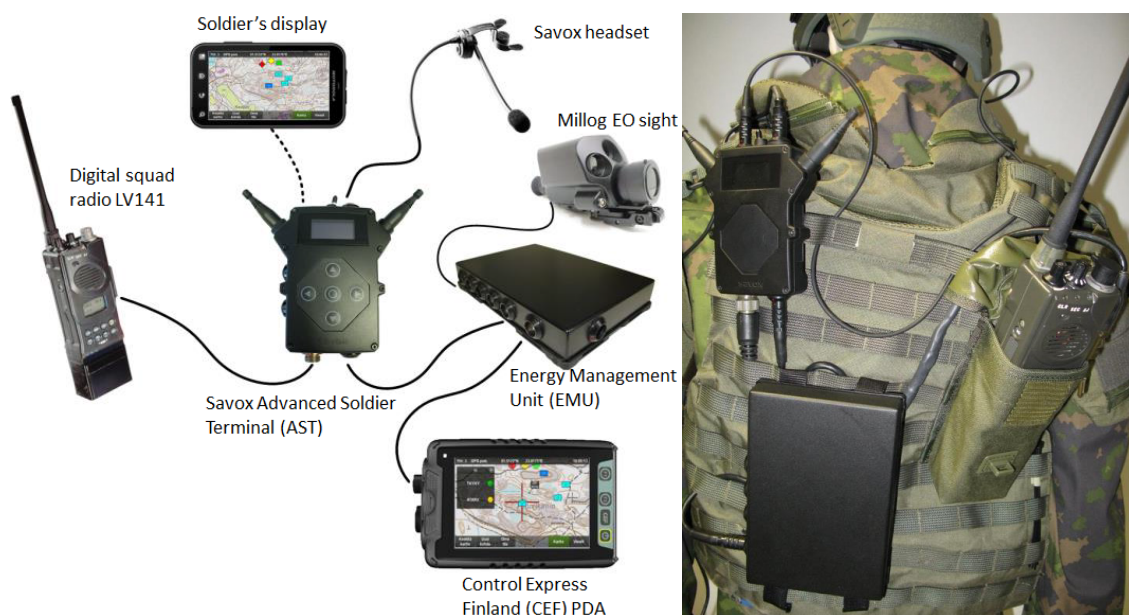
Figure 2-8: Electronic Power Management System Prototype for Dismounted Soldier with the Soldier's Display, Savox Headset, Millog EO Sight, Digital Squad Radio (LV141), Savox Advanced Soldier Terminal, Energy Management Unit and the Control Express Finland PDA [18].
