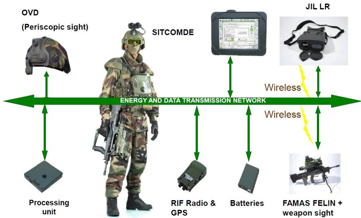
Figure 2-12: Energy and Data Transmission Network of the FÉLIN Soldier System [21].
